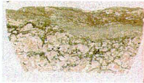
T2 15.10 Mylonite (top) Altered ÄD (bottom)
