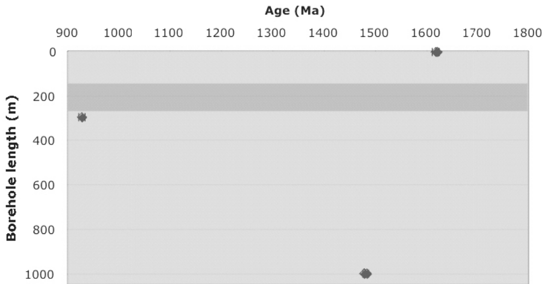
Figure 5-20. ^{40}\text{Ar}/^{39}\text{Ar} biotite age vs borehole length profile from KSH03A/B. The red band marks an identified deformation zone from the geological single-hole interpretation.
