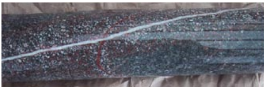
Figure 2-9. Drill core from KFM05A with sealed fractures. Image taken from /Sandström and Tullborg 2005/.
