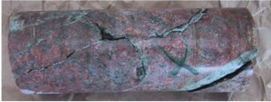
Figure 2-7. Fractures intersecting a drill core sample from KFM05A. Image taken from /Sandström and Tullborg 2005/.
