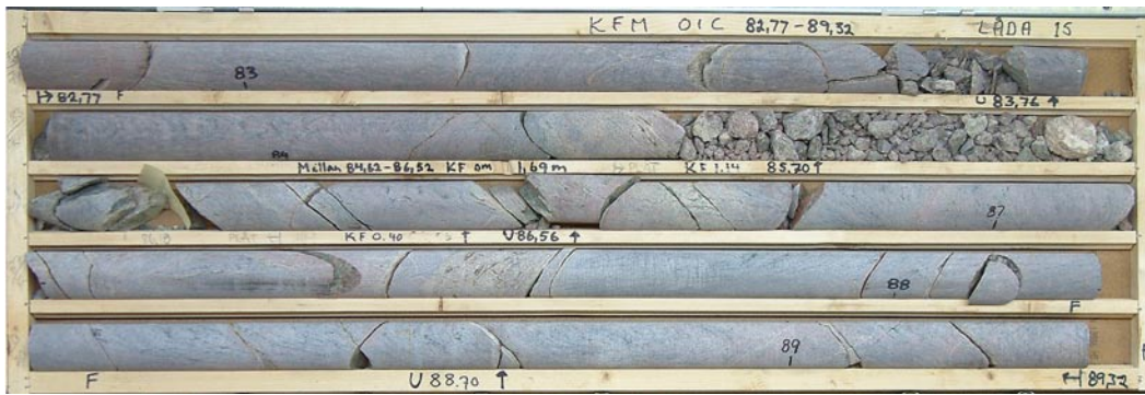
Figure 5-10. Drill core from instable section in borehole KFM01C.
