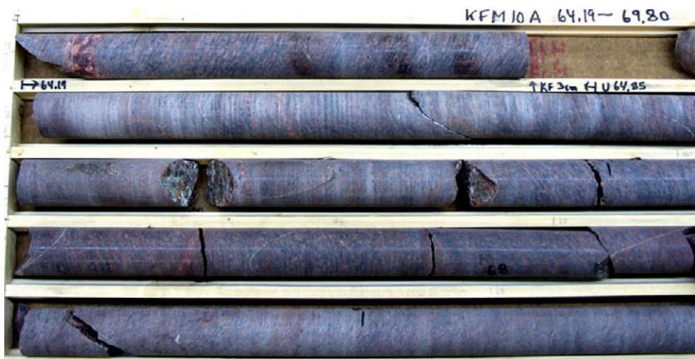
Figure 5-101. An overview of the upper part of DZ1 in KFM10A. A moderate frequency of single fractures coated with chlorite, clay minerals and minor calcite dominates.
