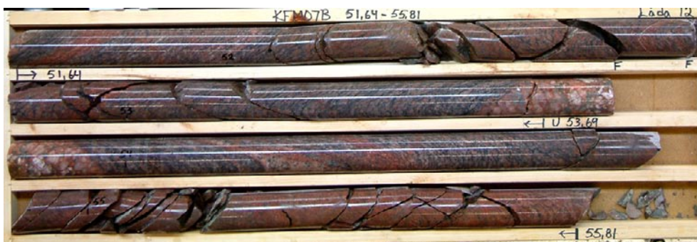
Figure 5-36. Photograph of the core in the upper part of DZ1. Note abundant fractures at 52–53 m and especially at 55–56 m. Photo: Alf Sevastik, SKB.
