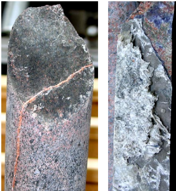
Figure 5-21. To the left: Thin NW-SE calcite-laumontite-quartz-sealed fracture at 127 m (pink colours on stereoplot in Figure 5-20) that cuts a chlorite-coated fracture. To the right: N-S calcite-fluorite-quartz-pyrite-filled fracture as an example of the few fractures present at the base of the DZ at 162 m (blue colour on stereoplot in Figure 5-20).
