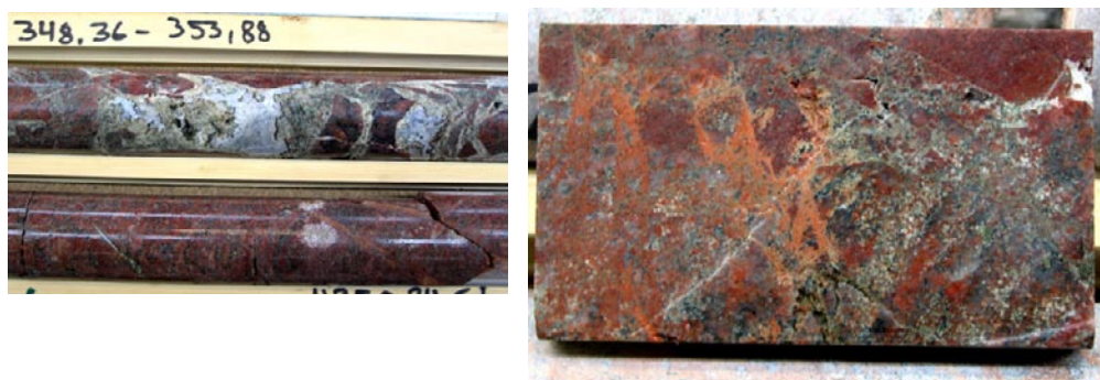
Figure 5-44. Left: Laumontite-cemented proto-breccia cut by a younger calcite- and prehnite-cemented breccia at 348.8 m. Right: The border between the two types of breccia and a thin vein that transect the laumontite-rich breccia (see details from thin section below).
