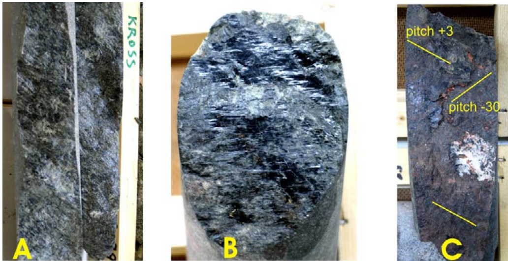
Figure 5-72. Examples of fault surfaces in KFM09A_DZ3. A. Polished surface with clays and chlorite and grooves, unknown sense of shear (strike/dip angle/pitch: 159/87/7) (265.03 m). B. Sinistral sense of shear with smooth and polished chlorite and clays (strike/dip angle/pitch: 329/84/10) (250.03 m). C. Two shears on the same fault surface: sinistral sense of shear with small steps and polished chlorite and hematite (strike/dip angle/pitch: 163/76/3) and undetermined oblique sense of shear with striae on chlorite and hematite (pitch: -30) (247.53 m).
