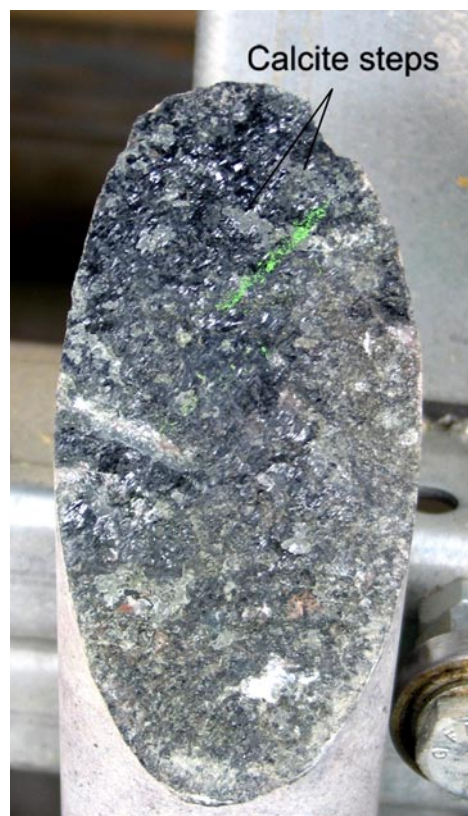
Figure 5-54. Left: Stereoplot of fault slip data in DZ2 (KFM08C). Right: Example of fault surface along DZ2 in KFM08C with sinistral steps of calcite and striations on chlorite (strike/dip angle/pitch: 204/71/-3) (537.19 m).
