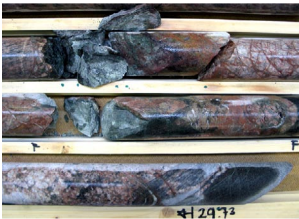
Figure 5-83. KFM09B_27.5 m. The drill core shows some hematite alteration, fractures are coated with chlorite, clay minerals and hematite, and there are some breccias sealed with chlorite + calcite + laumontite.
