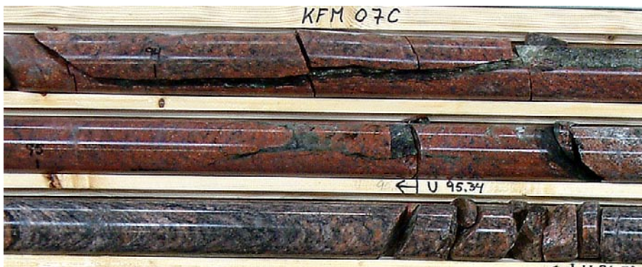
Figure 5-41. Overview of the brittle structures at the top of DZ1 in KFM07C. Steep chlorite-calcite filled fractures cut gently-dipping fractures filled with chlorite and clay minerals. Thin calcite-filled veins perpendicular to the drill core are also present.
