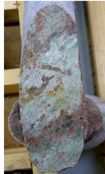
Figure 5-32. Left: Stereoplot of fault slip data along DZ3 in KFM06C. Right: Example of fault surface in KFM06C_DZ3 with striae on clay mineral and chlorite, unknown sense of shear (strike/dip angle/pitch: 328/73/-46) (454.47 m).
