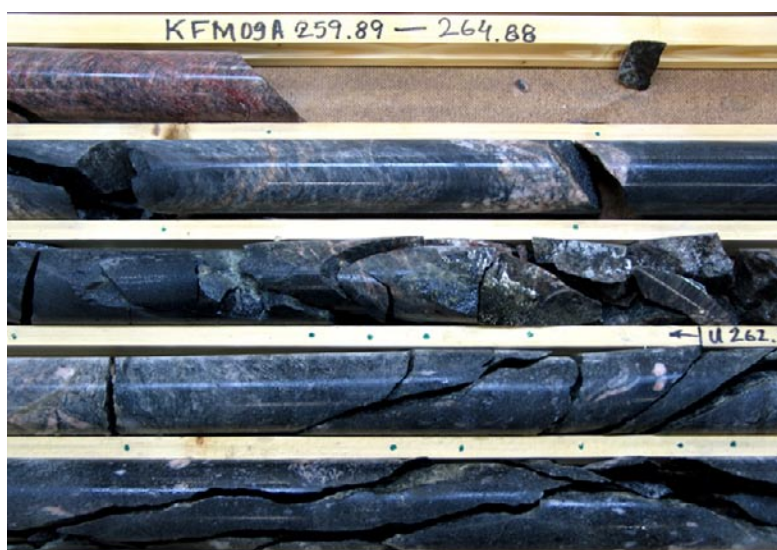
Figure 5-69. Increase of broken chlorite-calcite-filled fractures in the interval 262.5–264 m. The rock types are metagranite and some amphibolite.
