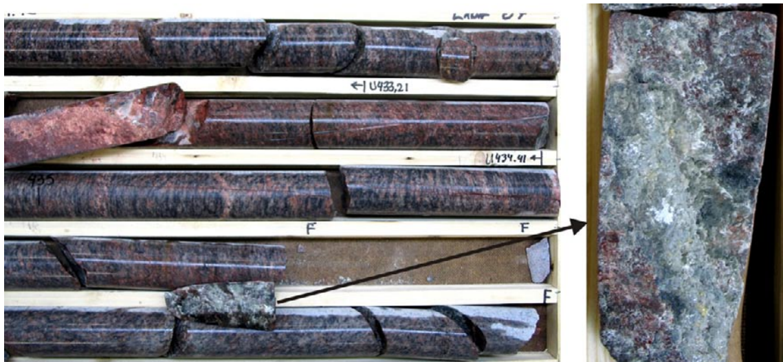
Figure 5-105. Left: Fractures with calcite-laumontite in grey metagranite-granodiorite that are oriented parallel to the drill core in DZ2 of KFM10A. Right: Example of fault plane with greenish calcite steps showing a reverse/sinistral sense of shear (strike/dip angle/pitch: 354/44/-26) (436.36 m).
