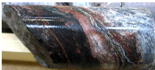
Figure 5-13. Photo showing highly sheared and oxidised mafic lithology and metagranites. A fault with striation (chlorite+hematite) occurs along the upper surface (to the left).
