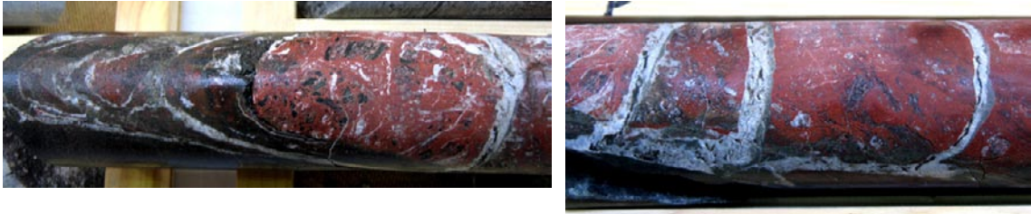
Figure 5-74. Left: A chlorite-laumontite-calcite-pyrite-sealed breccia (in green on picture) at the top of a laumontite-sealed breccia (at 732.5 m). Right: calcite-sealed veins cutting the laumontite-rich breccia.
