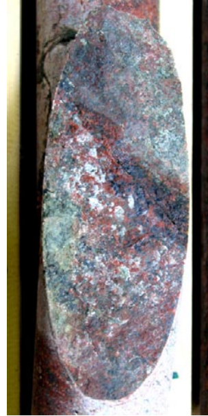
Figure 5-22. Left: Stereoplot of fault slip data along DZ1 in KFM06C. Right: Example of fault surface with striae on hematite and chlorite, and sinistral steps of calcite showing sinistral sense of slip (strike/dip angle/pitch: 185/82/0) (142.10 m).
