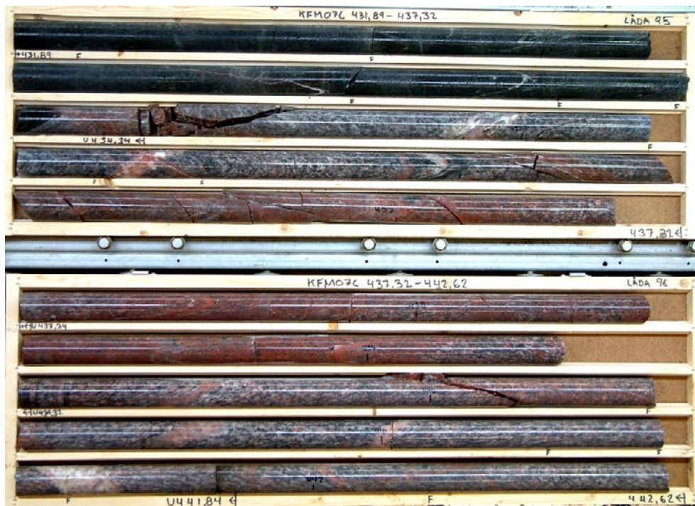
Figure 5-49. An overview of DZ3 in drill core KFM07C.
