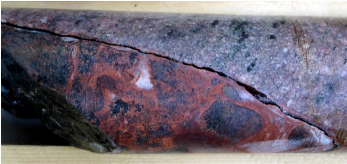
Figure 5-29. Laumontite- and adularia-rich brecciated zone at 429.50 m limited by two NE-SW chlorite-filled veins (the top most is plotted on the stereonet in Figure 5-28).
