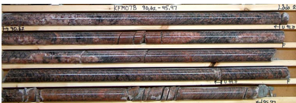
Figure 5-38. The upper part of DZ2 (92–95 m) exhibits moderate fracture frequency. Note relatively abundant open fractures at 95–96 m. A set of parallel laumontite-sealed fractures form a network at ca 93.5 m. Photo: Alf Sevastik, SKB.
