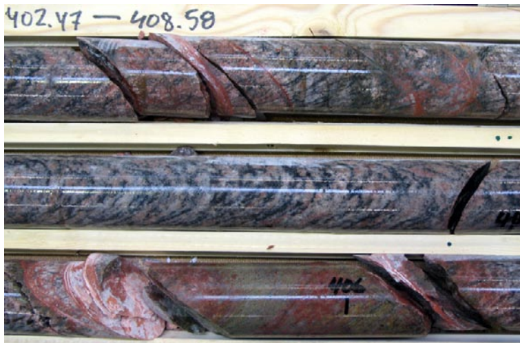
Figure 5-91. Photo of the drill core at ca 406 m showing an epidote-altered zone with quartz cut by a network of WSW-ENE steep fractures sealed with laumontite and calcite.
