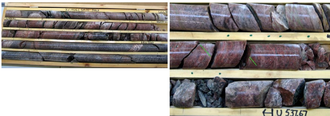
Figure 5-34. Left: notable increase in broken fracture frequency in the interval from 535 to 538 m, tentatively forming a fault core according to the definition of /Munier et al. 2003/. Right: an enlarged view of the picture to the left with the trend of the epidote-sealed veins underlined in green.
