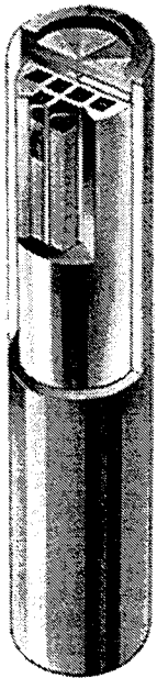
Figure 2.6 Copper canister with inner steel container
