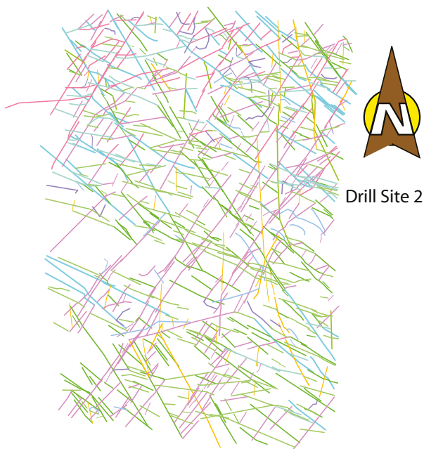
Figure 2-6. Fracture trace maps with different fracture sets identified in outcrop shown in different colours. Note the dominant Northwest-Southeast and Northeast-Southwest fracture sets.
