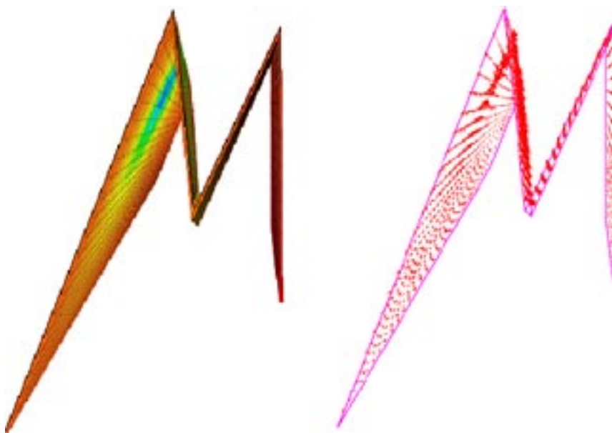
Figure 3-1. ANDRA-CEA detailed flow and transport model for structures 20–23 showing the head field (left) and the Darcy velocity field (right) /Grenier and Bernard-Michel 2006/.
