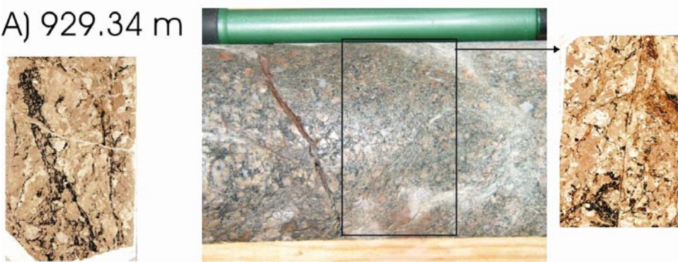
Figure 5-55. Samples of A) epidote rich cataclasite, B) cataclasite and C) chlorite rich cataclasite. Scanned thin sections of samples show A) a progressive fault rock evolution from cataclasite (top), to gouge (black), and ultracataclasite (bottom). B) Two generations of cataclastic reworking, and C) brittle micro-scale faults and a network of fine strands of ultracataclasite and gouge overprinting an older cataclasite.
