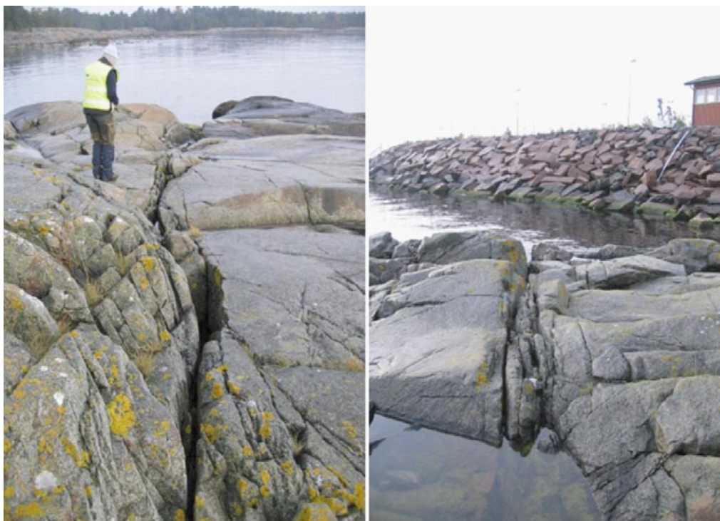
Figure 5-32. View to the north (left) and to the south (right) of the NS trending sinistral brittle fault. The person on the left stands between the main fault strand (in front of the person) and a prominent sinistral Riedel.
