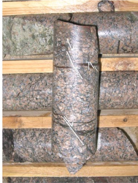
Figure 5-60. Orientation of fracture and fault planes (gently to moderately dipping great circles) and veins (subvertical planes) observed in KLX07A. The photograph shows subparallel normal and reverse faults cutting across thin gouge/ultracataclastic layers. A complex reactivation history is inferred.
