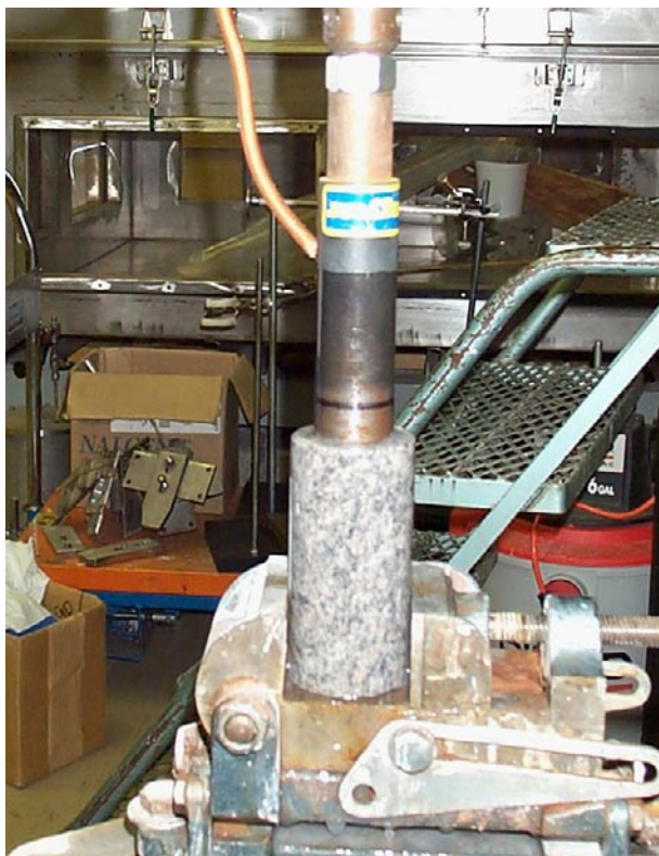
Figure 4-1. KFM01D core samples cut for permeability measurements.
