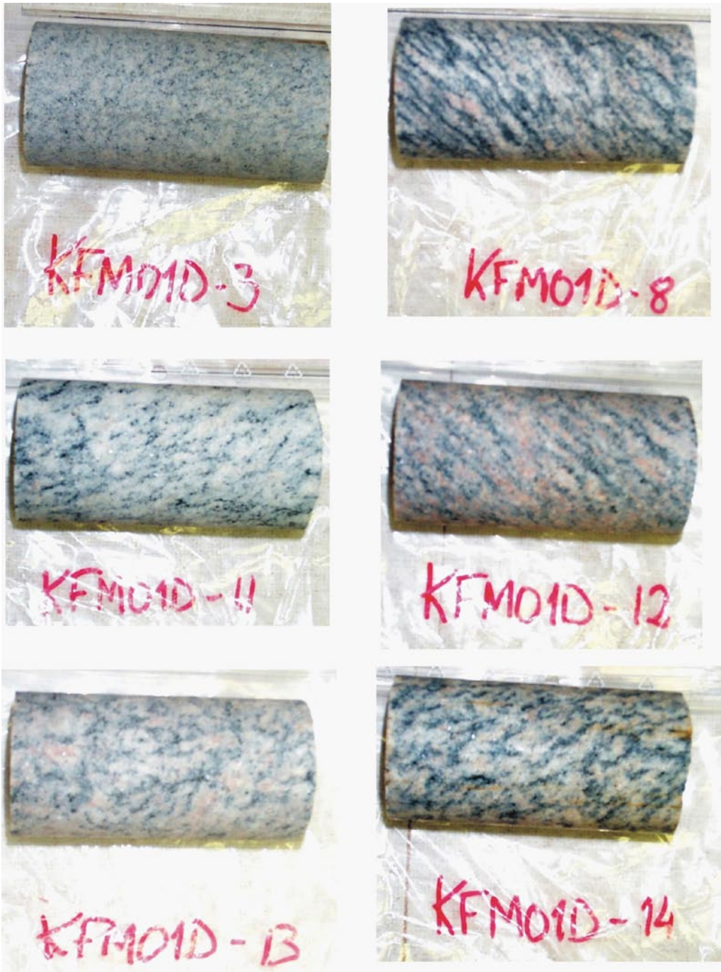
Figure 3-4. KFM01D core samples received from Geosigma.
