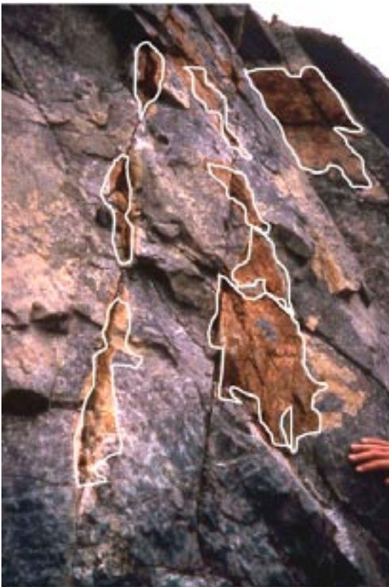
Figure 3-2. Channelling in the Poços de Caldas uranium mine seen as precipitates of iron oxides in the rock matrix into which oxygen has diffused and reacted with pyrite. White lines have been drawn around the oxidized red rock. The grey rock has not been invaded by oxidizing waters.
