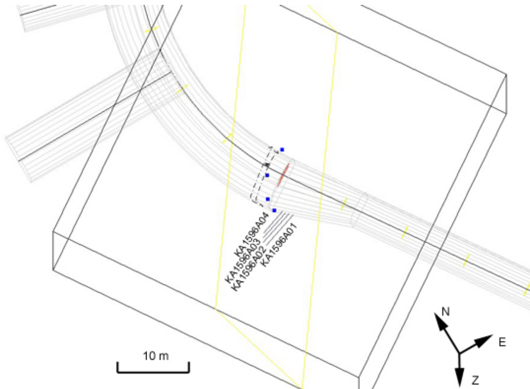
Figure 6-1. Visualization of the points (blue) based on tunnel survey and used for the remodeling of 'zone 1600', and positions of the boreholes.
