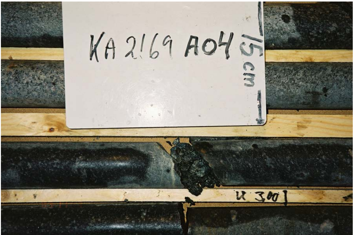
Figure A1-6. Fault in KA2169A04 at 3 m borehole length.
