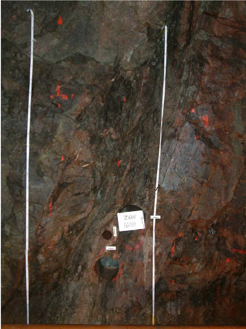
Figure A1-10. Target fault zone at tunnel section 1/600 m.
