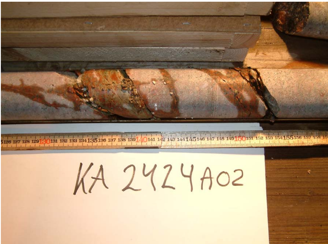
Figure A1-3. Fault at 2.5 m in KA2424A02 drill core.
