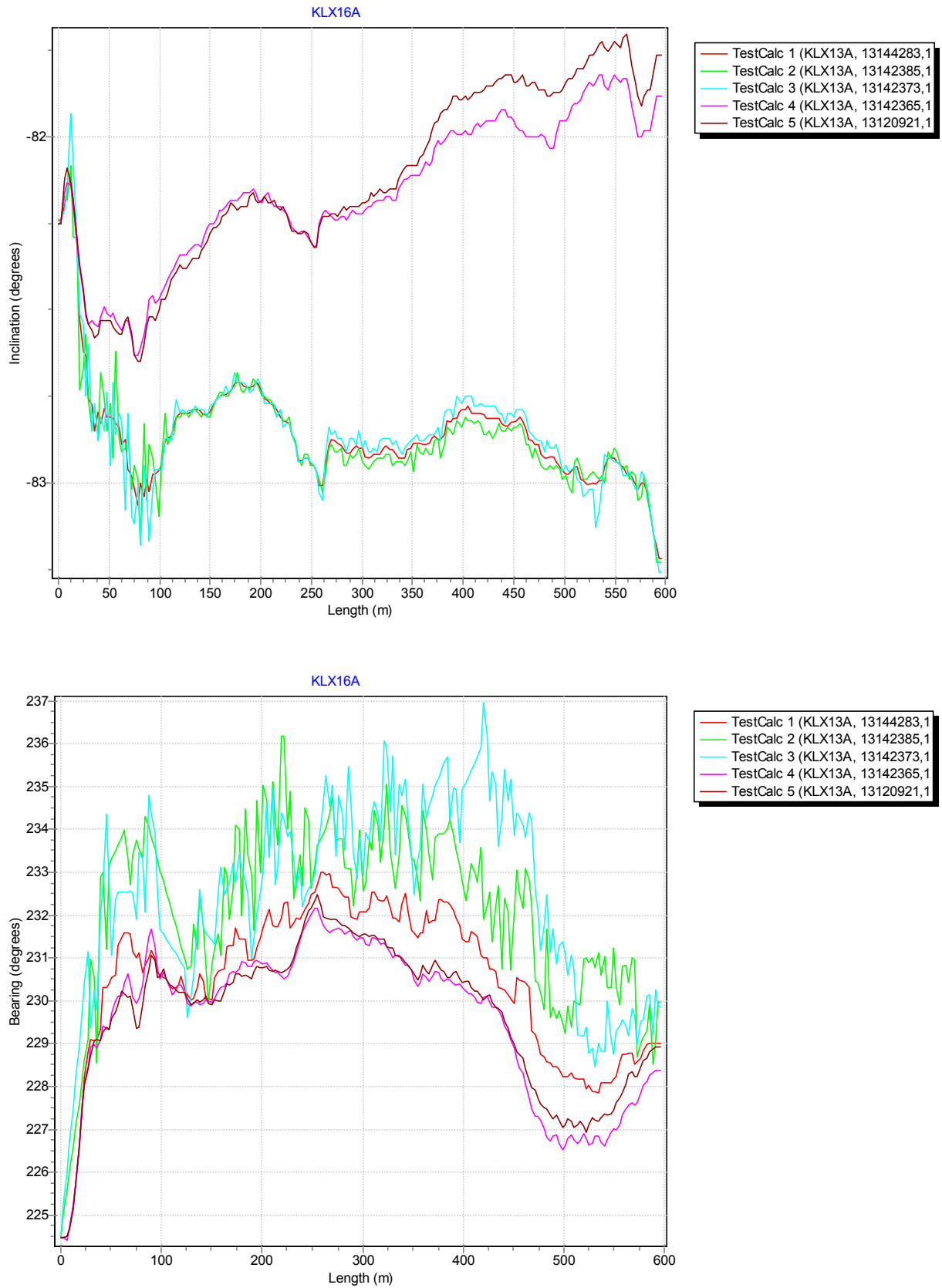
Figure 4. The Borehole deviation multiple measurements data (red line) together with the other, not ERROR- marked, deviation activities specified in Table 1. The upper diagram shows the inclination and the lower shows the bearing.
