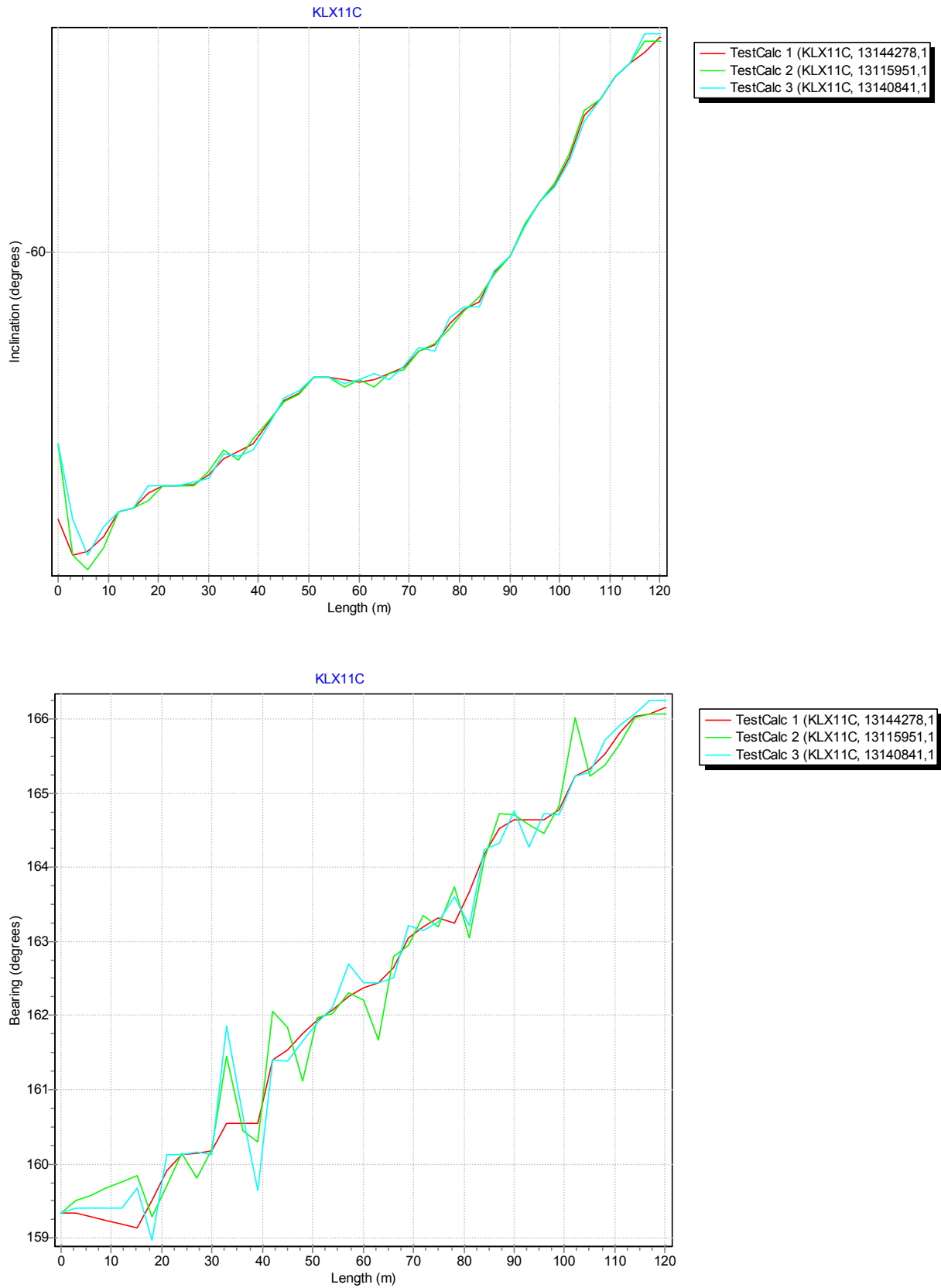
Figure 3. The Borehole deviation multiple measurements data (red line) together with the other, not ERROR- marked, deviation activities specified in Table 1. The upper diagram shows the inclination and the lower shows the bearing.
