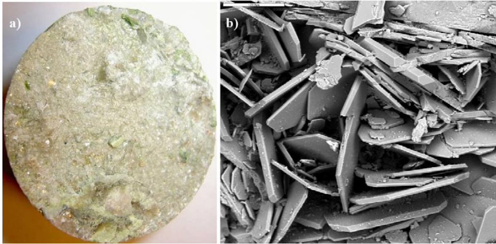
Figure 7-8(a-b). a) Photograph of an open fracture, mainly coated with apophyllite. b) Back-scattered SEM-image of apophyllite from the fracture surface in figure a. Scale marker is 200 \mu\text{m} . Sample KLX03: 970.04–970.07 m.
