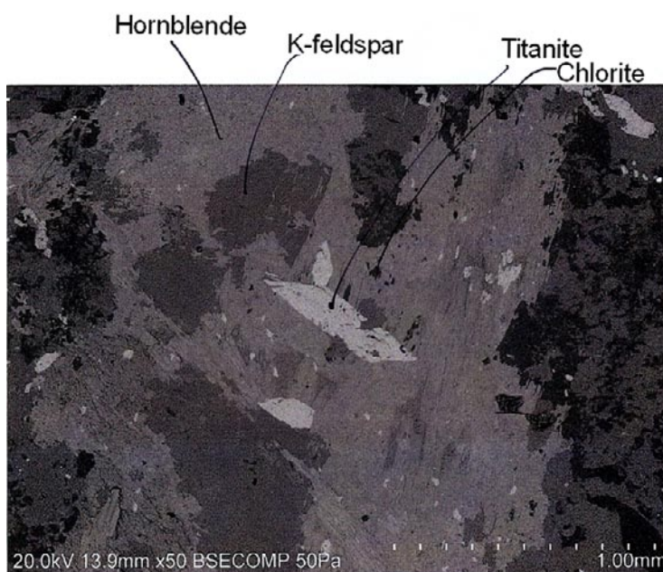
Back-scattered SEM-image showing the sealed fracture. The titanite crystals may originate from the wall rock. Sample KLX08: 933.15–933.30 m.
