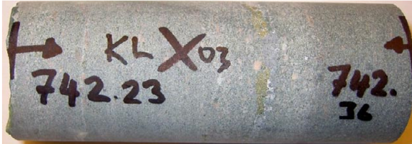
Photograph of the drill core sample KLX03: 742.23–742.36 m showing a fracture filled with quartz, pyrite, calcite and chlorite.
