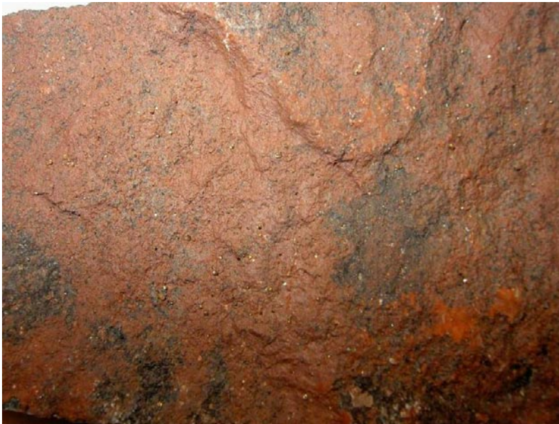
Photograph of the drill core KLX04: 673.78–674.05 m showing hematite (red) and pyrite (small crystals) on the surface of the open fracture.
