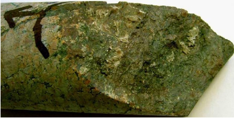
Photograph of the fracture surface KLX07A: 557.83–557.94 m. Bladed calcite is visible.
