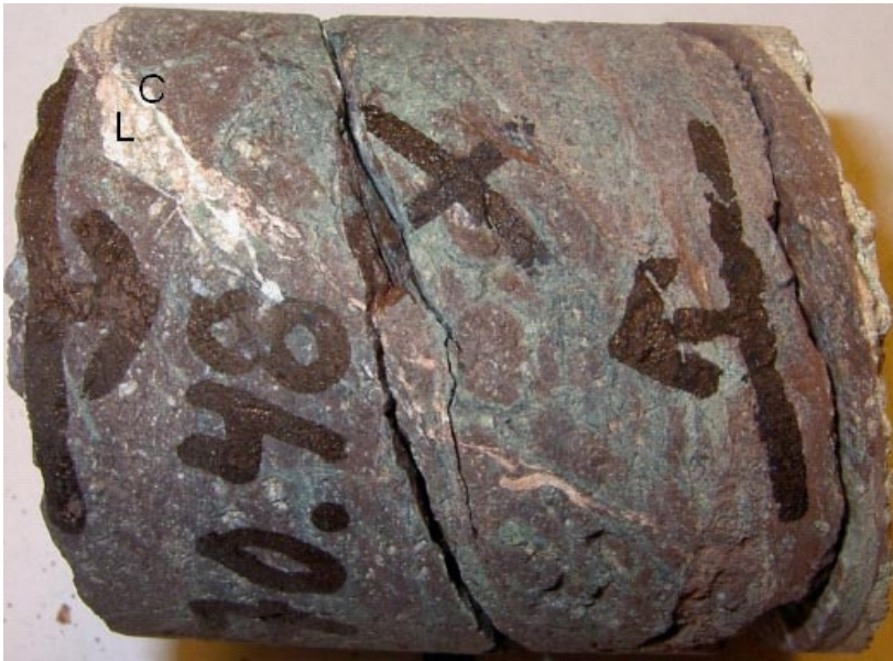
Photograph of the drill core KLX04: 970.48–970.52 m showing cataclasites (one brown and one green variety) cut by a laumontite-filled fracture (L) which is cut by a calcite-filled fracture (C).
