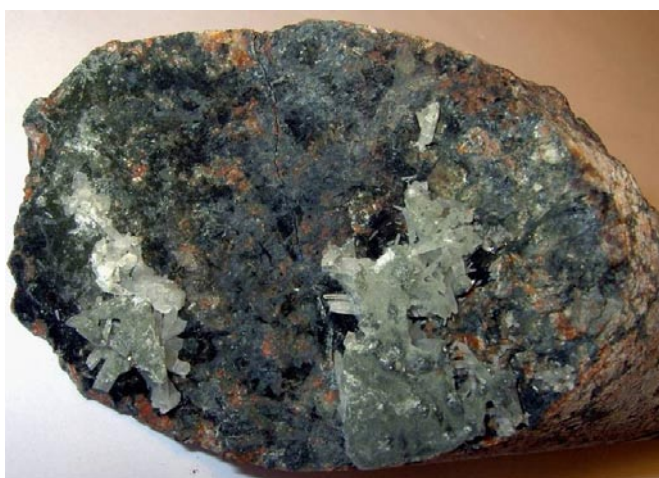
Photograph of the fracture surface KLX08: 108.24–108.33 m. Dark green parts are dominated by chlorite and clay minerals while the bright parts are dominated by needle shaped calcite.
