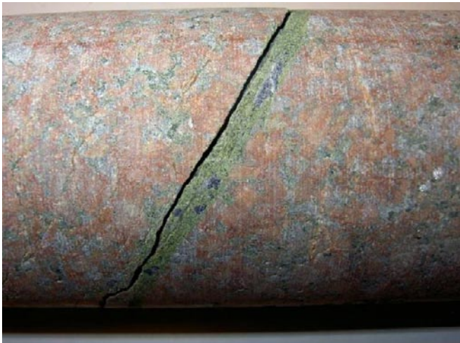
Photograph of the drill core KLX04: 188.19–188.39 m showing a fracture filled with epidote (green) and fluorite (purple).
