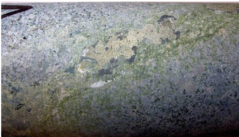
Photograph of the sealed fracture KLX08: 676.92–677.13 m.
