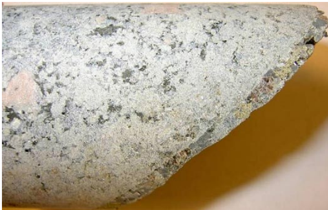
Photograph of the drill core KLX06: 590.66–590.72 m. The coating is made up of muscovite, pyrite, quartz and fluorite.
