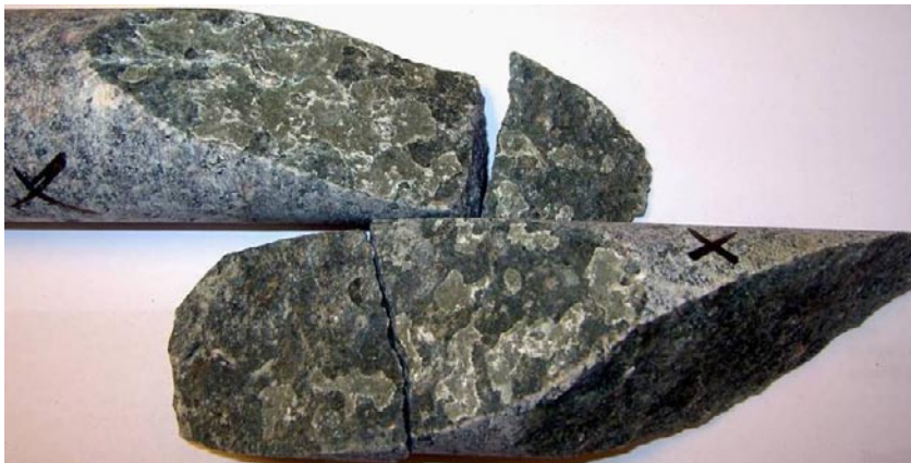
Photograph of the fracture surfaces. Sample KLX08: 795.15–795.36 m.
