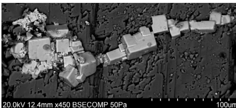
Back-scattered SEM-image of pyrite on top of calcite. Sample KLX07A: 373.70–373.97 m
