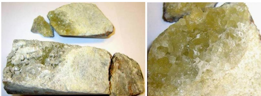
Photographs of the drill core sample showing the fracture coating that is dominated by fluorite (yellow) and whitish calcite. Drill core diameter is 50 mm. Right photograph is a close-up of the fluorite rich part. Sample KLX06: 814.86–814.95 m.
