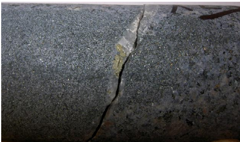
Photograph of the drill core KLX03: 591.33–591.33 m showing a re-activated fracture originally sealed by quartz and pyrite. Drill core diameter is 50 mm.
