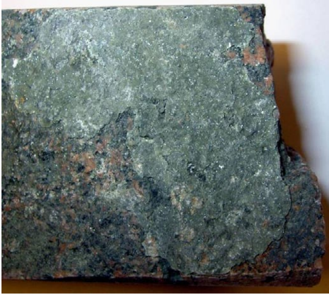
Photograph of the fracture surface KLX10A: 610.85–611.19 m. The glittering crystals are apophyllite. The green colour comes from corrensite.
