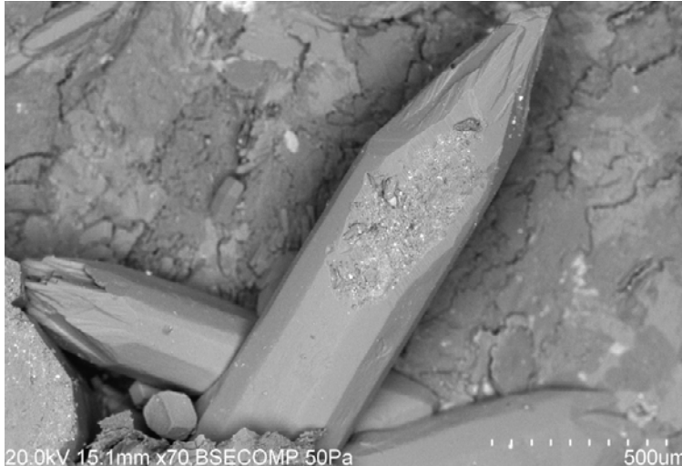
Back-scattered SEM-image of needle shaped calcite. Sample KLX08: 218.29–218.39 m.
