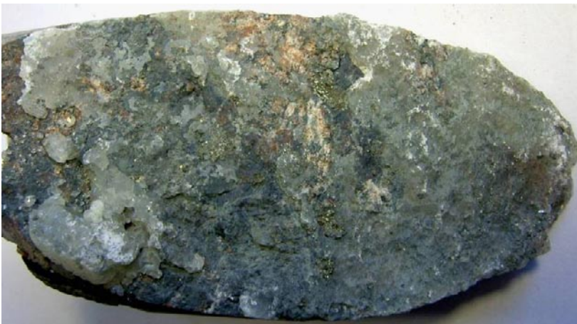
Photograph of the fracture surface KLX07A: 668.98–669.22 m. Calcite and pyrite is visible.
