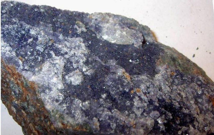
Photograph of the drill core KLX04: 925.60–925.68 m showing fluorite (purple) and calcite (white) on the surface of the open fracture.
