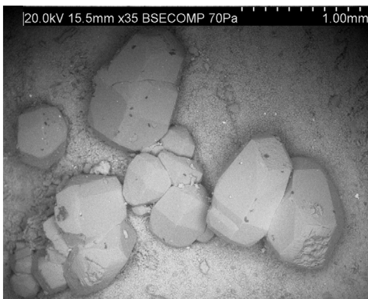
Back-scattered SEM-image of equant calcite crystals (KLX07A: 696.68–696.83 m).
