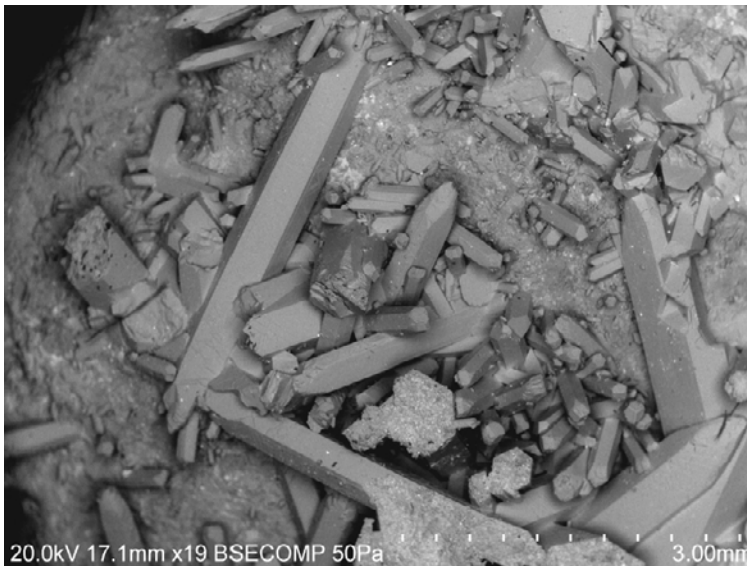
Back-scattered SEM-image of needle shaped calcite. Sample KLX08: 218.29–218.39 m.
