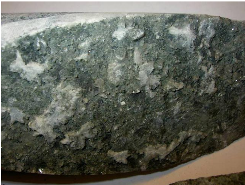
Photograph of the drill core KLX04: 669.31–669.55 m showing the surface of the open fracture. Drill core diameter is 50 mm.
