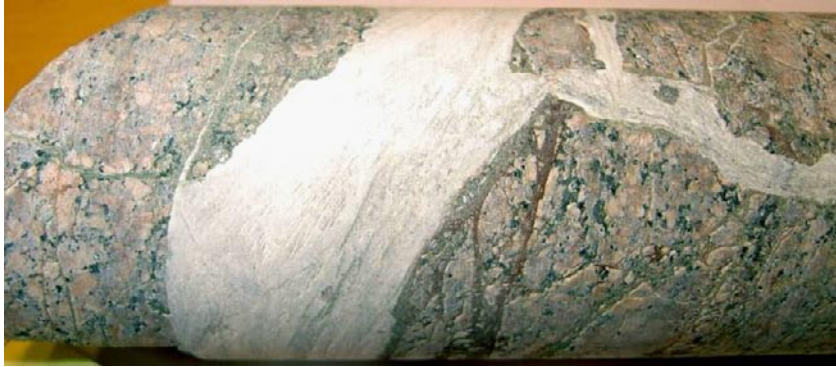
Photograph of the sealed, calcite-filled, fracture, which cuts through cataclasite (dark red-brown). Sample KLX08: 478.87–479.13 m.
