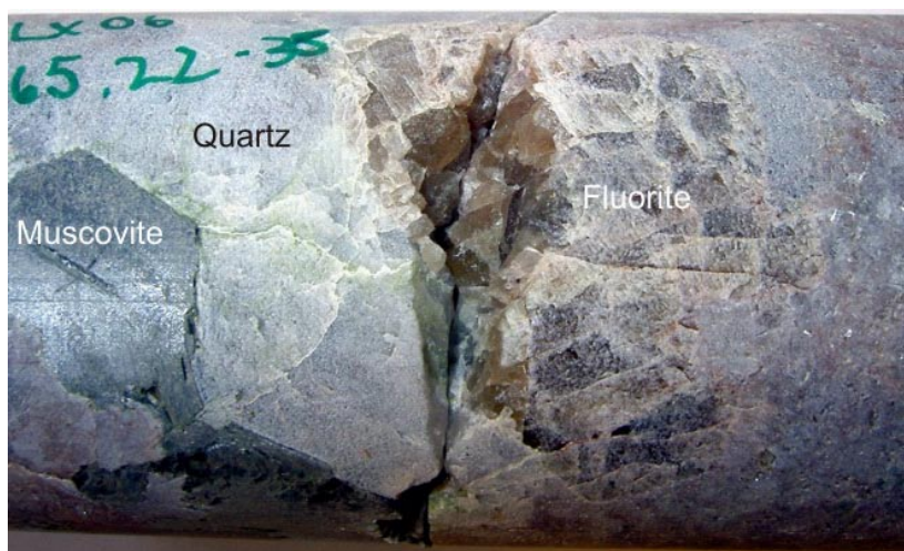
Figure 7-16. Photograph of coarse-grained muscovite, quartz and fluorite in sample KLX06: 565.22–565.38 m.
