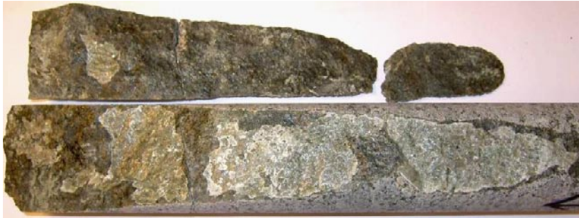
Photograph of the fracture surfaces. Sample KLX08: 792.43–792.72 m.
