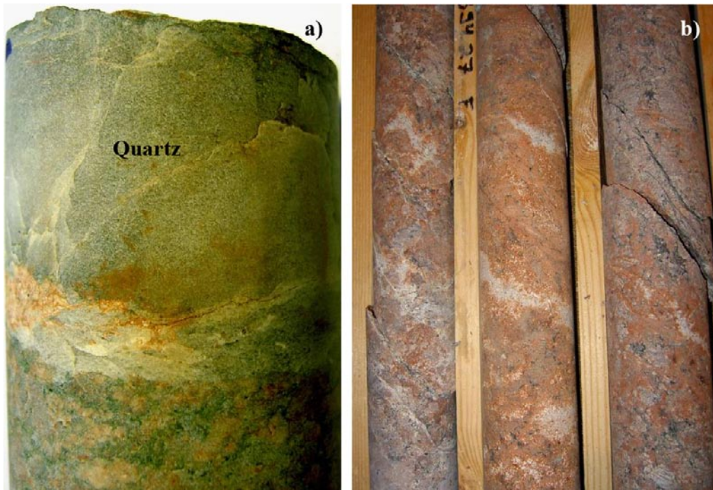
Figure 7-5(a-b). a) Photograph of quartz, calcite (whitish grey, lower part of the filling), and laumontite (orange). Sample KLX07A: 106,25–106,41 m. b) Photograph of parts of the laumontite-rich zone in KLX06 (392–394 m).
