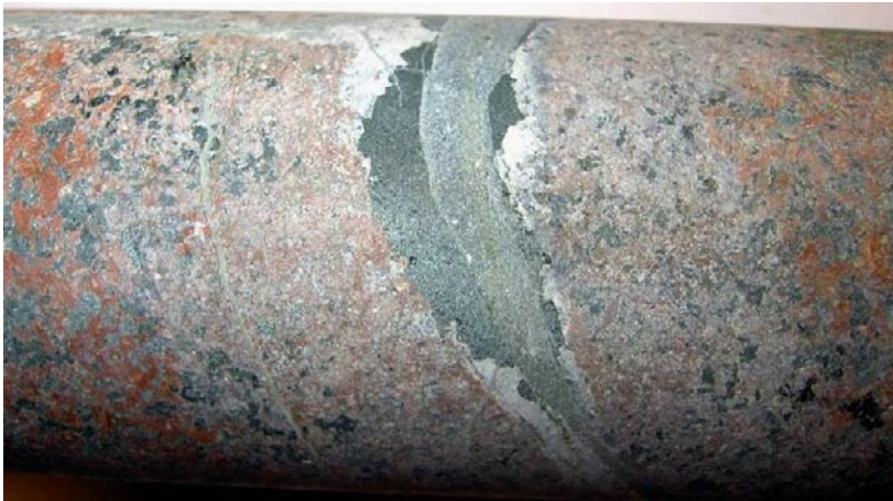
Photograph of the drill core KLX03: 722.72–722.96 m showing a fracture filled with chlorite, calcite and quartz that is cut by a fracture filled with predominantly prehnite. Note the shifting colouration of the wall rock towards the fracture.
