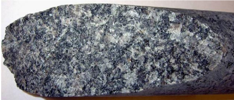
Photograph of the drill core KLX03: 572.10–572.30 m showing the fracture surface partially covered with gypsum. Drill core diameter is 50 mm.
