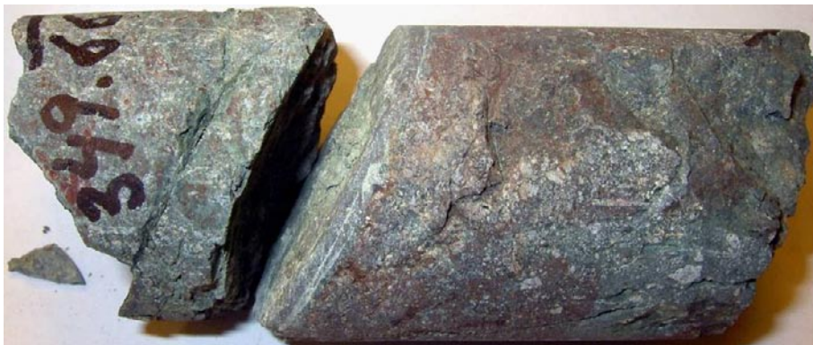
Figure 7-1. Photograph of drill core sample KLX04 349.66–349.79 m that shows red-brown coloured cataclasite cut by later formed fractures. The green-coloured cataclasite type is found in the left part of the sample.
