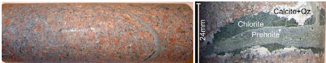
Figure 7-3(a-b). a) Photograph of a fracture filled with prehnite. The wall rock is hydrothermally altered and red-stained. Sample KLX08: 366.43–366.58 m. b) Photograph of prehnite (generation 4) in a fracture cutting through earlier formed chlorite, calcite and quartz (generation 3). Sample KLX03: 722.72–722.96 m.
