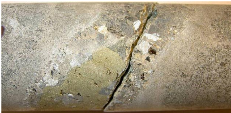
Figure 7-15. Photograph “greisen-like” alteration and coarse-grained pyrite and muscovite. Sample KLX06: 535.10–535.26 m.
