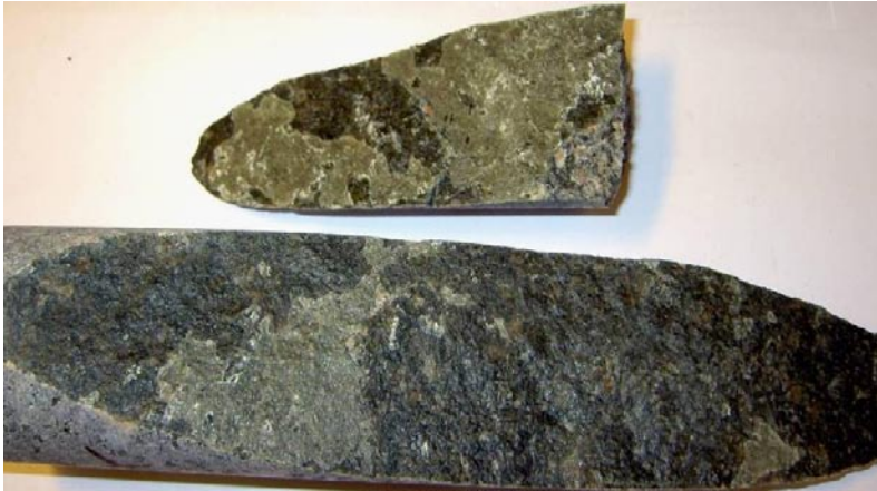
Photograph of the fracture surfaces. Sample KLX08: 820.93–821.16 m.
