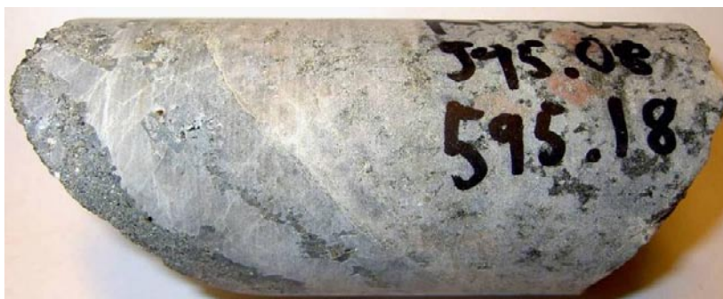
Photograph of the drill core KLX06: 595.08–595.18 m. Visible is muscovite and quartz.
