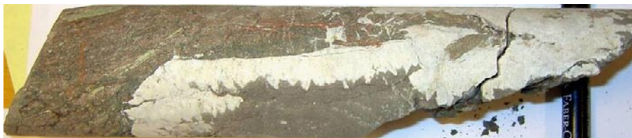
Photo of the sample KLX08: 772.49–772.69 m. Calcite in white and cataclasite in brown.
