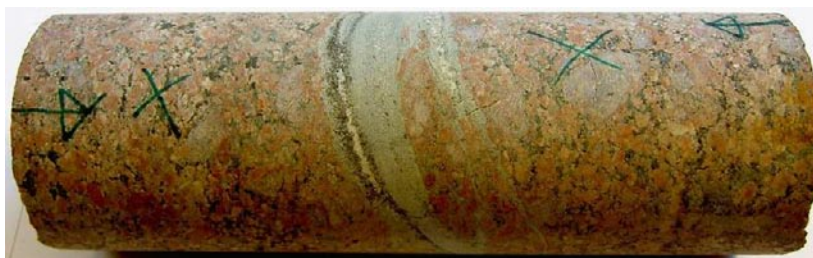
Photograph of sealed fractures filled with prehnite (bluish grey), calcite (white) and chlorite (dark). Sample KLX07A:227.24–227.38 m.
