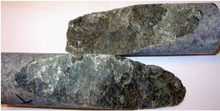
Photograph of the fracture surfaces. Sample KLX08: 916.16–916.36 m.
