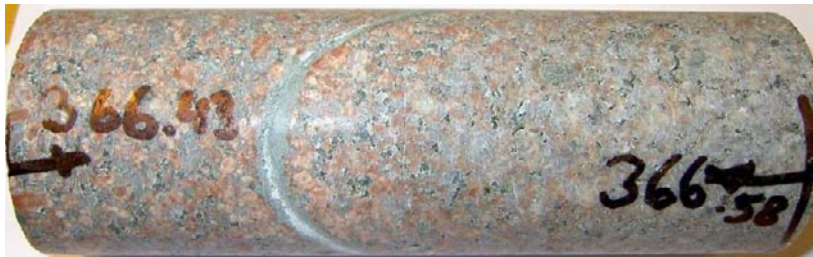
Photograph of the sealed fracture KLX08: 366.43–366.58 m. Prehnite in bluish grey and calcite in white.
