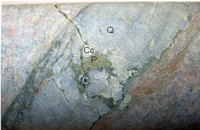
Photograph of the sealed fracture KLX07A: 423.21–423.39 m (Q = quartz, Cc = calcite, P = pyrite, C = chlorite).
