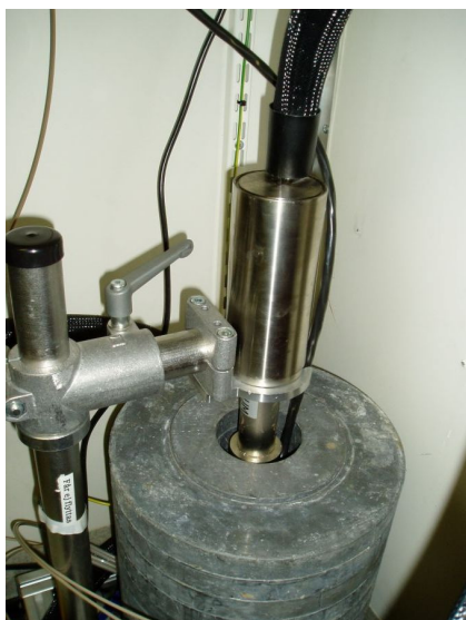
Figure 7. Lead shield and parts of the HPGe-detector used for on-line radioactivity concentration measurements.
