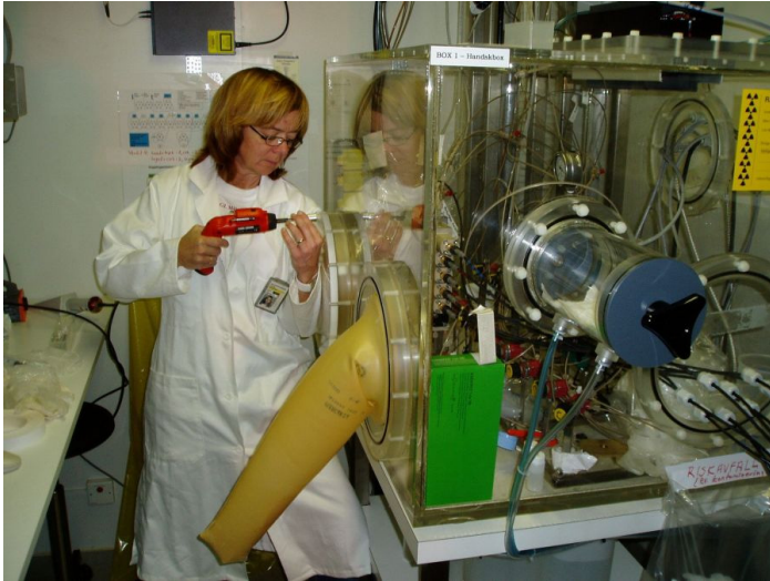
Figure 5. Inert gas glove box for all circulation equipment excluding the pressure regulator which is contained within a separate inert gas box.
