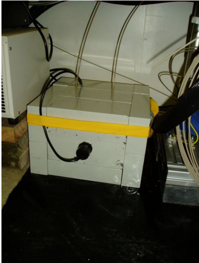
Figure 8. Lead shield and back part of the GM-probe used for on-line dose rate monitoring.
