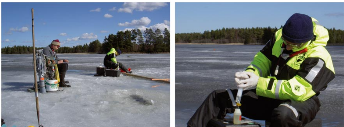
Figure 5-1. Left: Sampling of surface water from below wet and soft ice (Lake Bolunds-fjärden, April 2006). Right: Filtration of water in the field using a disposable filter.
