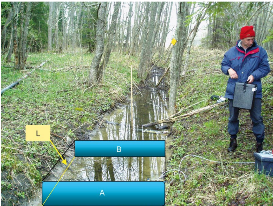
Figure 5-3. Schematic presentation for estimating water runoff in natural stream waters (see text for explanation). Sampling location PFM000073 (Söder Bredviken).
