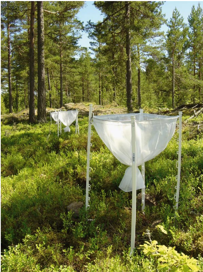
Figure 3-1. Annual litterfall from trees was measured using litter traps.
