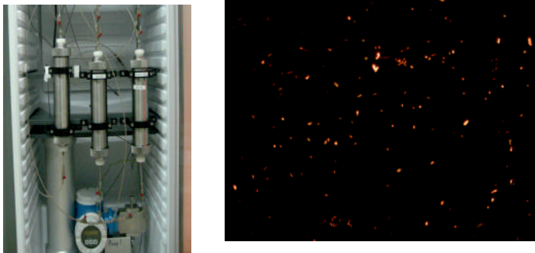
Figure10. (left) Reactors at the MICROBE site (Äspö HRL) for biofilm generation on different mineral slides. (right) Fluorescence microscopy snapshot of biofilm produced.
