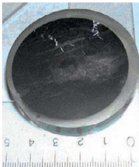
Figure. 2. Photograph of the bore core sample for testing in break through experiment
