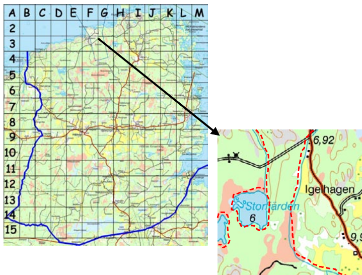
Figure 2-6. Principle for sampling of tracks crossing transects oriented along the water system. The red dashed lines indicate transects.
