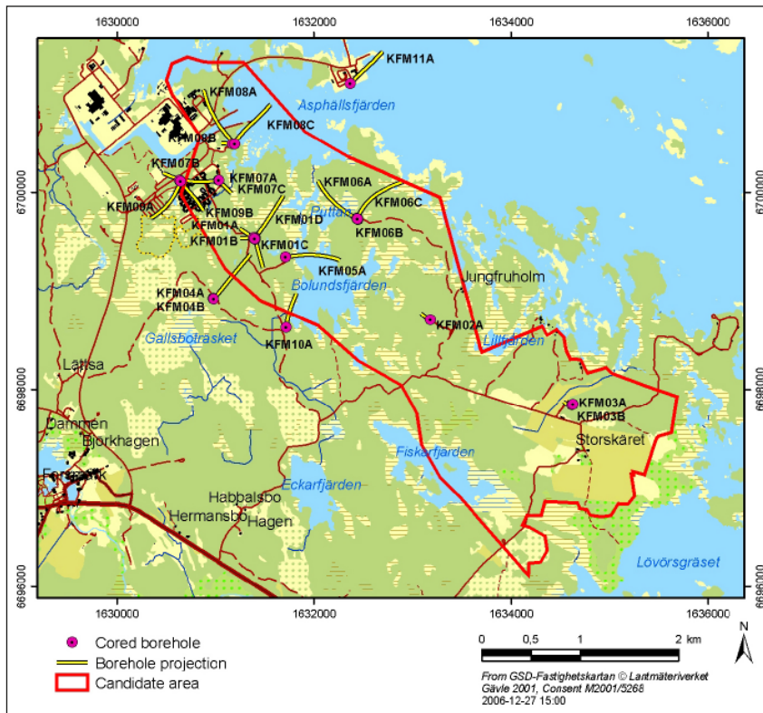
Figure 1-1. The investigation area at Forsmark (approximately the area shown) with the candidate area selected for more detailed investigation. The current telescopic and conventional core drilled boreholes are marked with pink filled circles.
