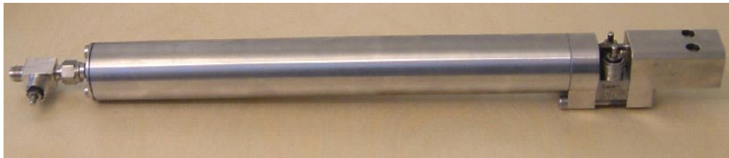
Figure A7-3. SKB stainless steel sampling cylinder, (left: piston side, right: mounting adapter side).
