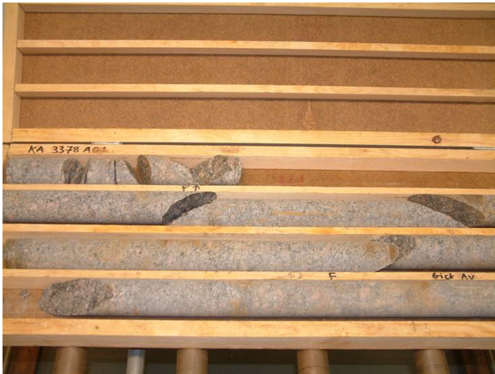
Figure 2-6. Borehole H (KA3378A01). Upper: Axial section of the borehole that intersects borehole G at the lower end. Lower: The core photo, with the upper part of the core at the upper left, shows that the rock around the upper end of the hole is strongly fractured but that the rest is intersected by only a few presumably water-bearing fractures. The hole has an average spacing of presumably water-bearing fractures of 0.5 m. A plug of “Container” type was inserted in the hole.
