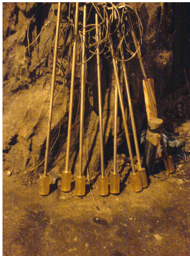
Figure4-3. Mechanical packers for sealing the plugged holes.
