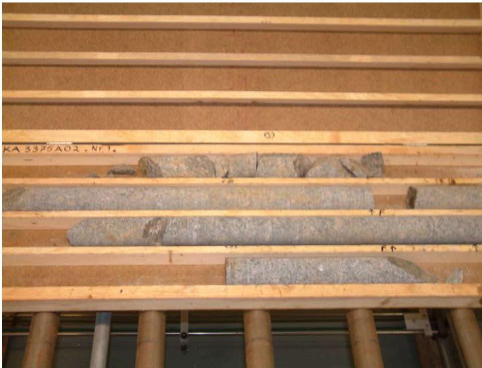
Figure 2-3. Borehole B (KA3375A02). Upper: Axial section of the borehole that intersects borehole A at the lower end. Lower: The core photo, with the upper part of the core at the upper left, shows that the rock has rather few fractures but that core loss took place where the A - and C -fractures ( A is a small zone) were intersected. The hole has an average spacing of presumably water-bearing fractures of 0.75 m. A plug of “Basic” type was inserted in the hole.
