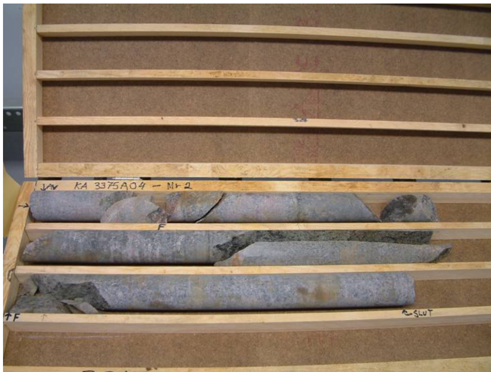
Figure 2-4. Borehole D (KA3375A04). Upper: Axial section of the borehole that intersects borehole C at the lower end. Lower: The core photo, with the upper part of the core at the upper left, shows that the rock is intersected by two major fractures interpreted as C and D . The hole has an average spacing of presumably water-bearing fractures of 0.5 m. A plug of “Pellet” type was inserted in the hole.
