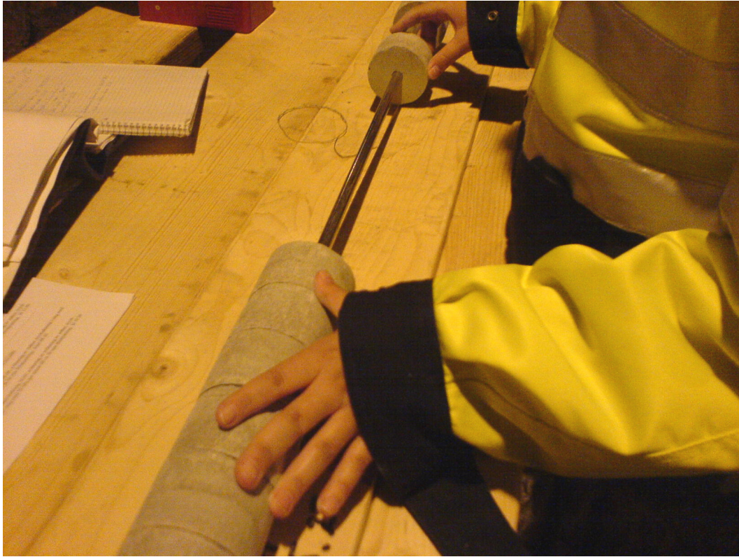
Figure 4-5. Preparation of the plug of Couronne Type in Hole E. The blocks are being stacked around the central rod.
