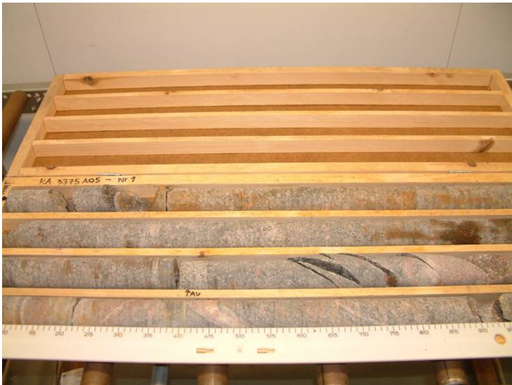
Figure 2-5. Borehole E (KA3375A05). Upper: Axial section of the hole which intersects borehole F at the lower end. Lower: The core photo, with the upper part of the core at the upper left, shows that the hole is intersected by a fracture zone at about 2.5 m distance from the top. Above the zone the rock is poor in fractures. The hole has an average spacing of presumably water-bearing fractures of 0.75 m. A plug of “Couronne” type was inserted in the hole.
