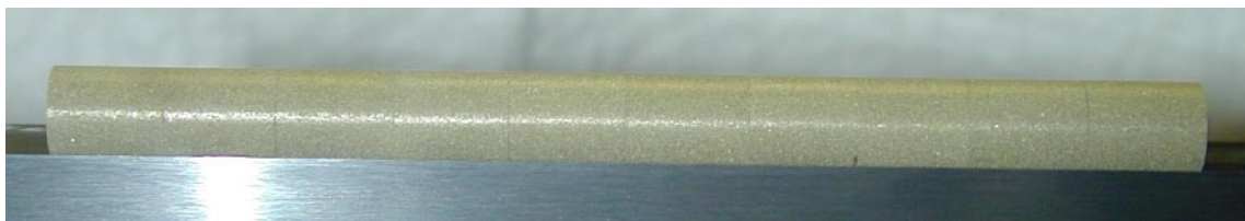
Figure 3-3. (Pu,Zr)N fuel pellets fabricated at PSI following a procedure suggested by KTH.
