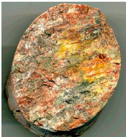
Striated open fracture with mainly clay minerals. The diameter of the drill core is c 5 cm.
