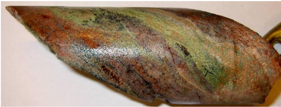
Figure 5-3. Altered rock with epidote. KFM07A 815.27–815.37 m. The diameter of the drill core is c 5 cm.
