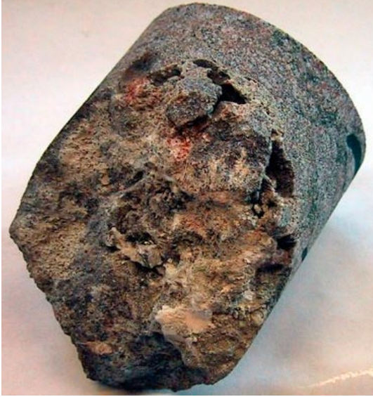
Open fracture coated with mainly quartz, adularia, illite and chlorite (orientation 145/36°). The diameter of the drill core is c 5 cm.
