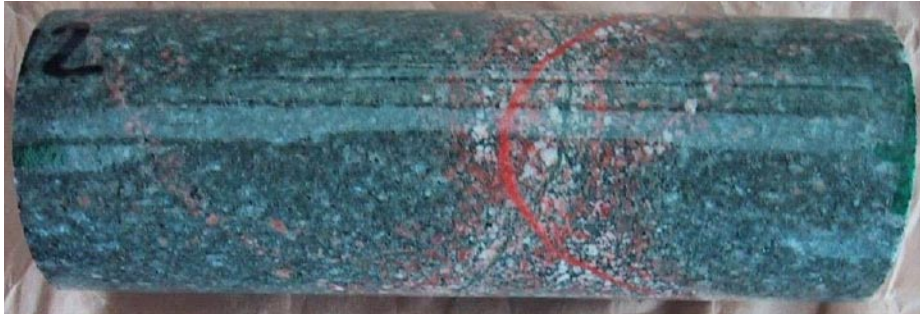
Figure 5-5. Epidote sealed fracture cut by a sealed fracture filled with hematite stained adularia. KFM05A 692.00–692.15 m. The diameter of the drill core is ~ 5 cm /Sandström and Tullborg 2005/.
