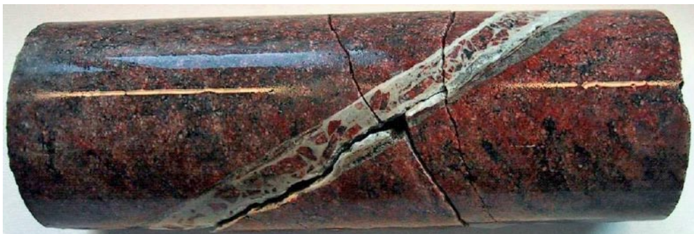
Figure 5-13. Prehnite sealed fracture and cut by a breccia sealed with a mixture of extremely fine-grained quartz and calcite together with larger calcite crystals. KFM08A 107.42–107.57 m. The diameter of the drill core is c 5 cm.
