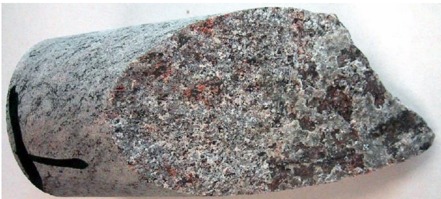
Figure 5-21. Open fracture with a thin precipitate of calcite, KFM08B 97.37–97.43 m. The diameter of the drill core is c 5 cm.
