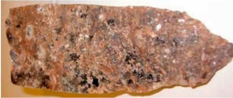
Open fracture with black spots consisting of iron oxide. The diameter of the drill core is c 5 cm.
