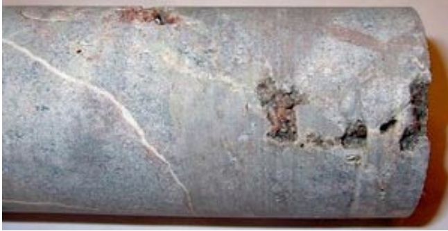
Thin fracture sealed with calcite. The diameter of the drill core is c 5 cm.
