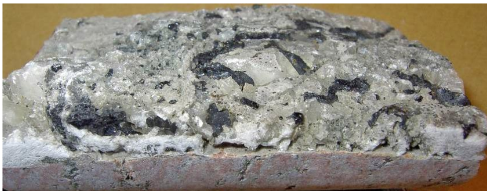
Figure 5-18. Black asphaltite in fracture together with calcite, quartz and pyrite, KFM06C 103.19–103.28 m. The diameter of the drill core is c 5 cm.
