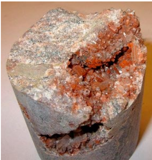
Open void with large euhedral crystals of quartz and adularia – red-stained of hematite. The diameter of the drill core is c 5 cm.
