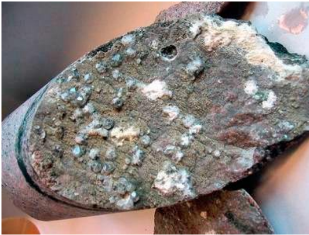
Open fracture coated with quartz and adularia on which euhedral crystals of pyrite and analcime have precipitated. The diameter of the drill core is c 5 cm.
