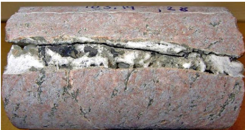
Partly open fracture with a mixture of euhedral calcite, small euhedral quartz crystals, asphaltite and small pyrite crystals.
