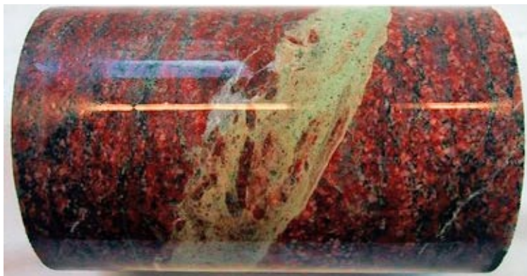
Epidote and calcite sealed fracture. The diameter of the drill core is c 5 cm.
