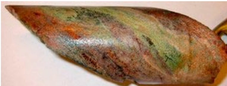
Altered wall rock of mainly saussuritized plagioclase and epidote. The diameter of the drill core is c 5 cm.
