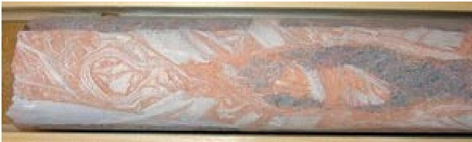
Sealed fracture with laumontite and calcite. The diameter of the drill core is c 5 cm.
