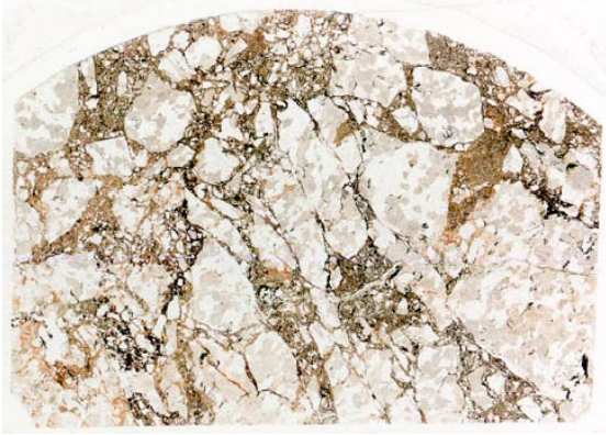
Scanned thin section of breccia sealed with quartz, adularia, chlorite, hematite and titanite. The base of the figure is c 35 mm.
