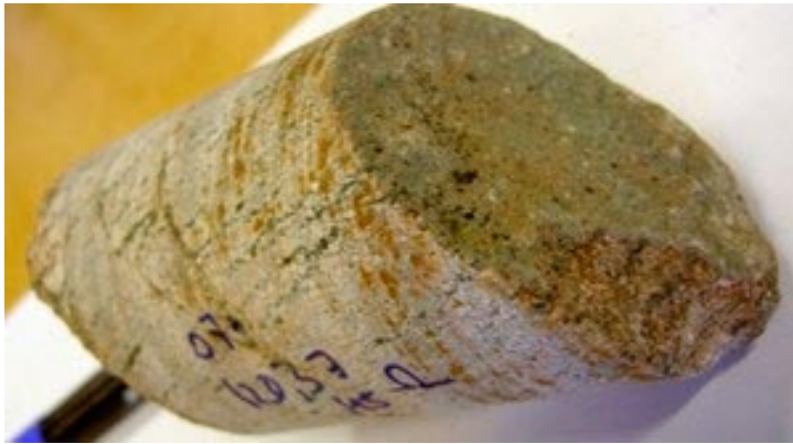
Open fracture with thin greenish coating of quartz, adularia, pyrite and an unidentified Zn-silicate (small black spots). The diameter of the drill core is c 5 cm.
