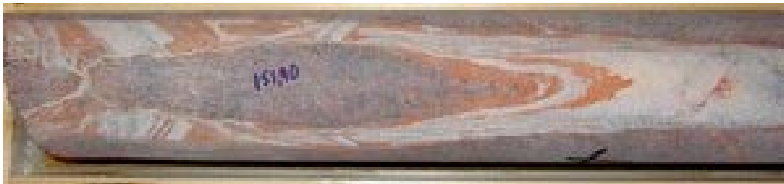
Sealed fracture with laumontite and calcite. The diameter of the drill core is c 5 cm.
