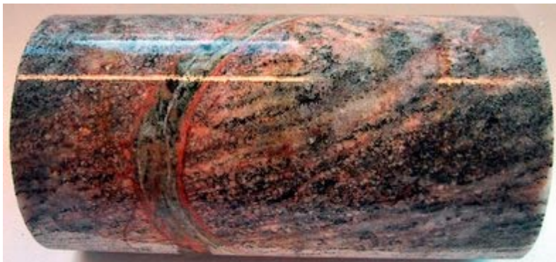
Sealed fracture with adularia, quartz, fluorite, hematite, prehnite and calcite. The diameter of the drill core is c 5 cm.
