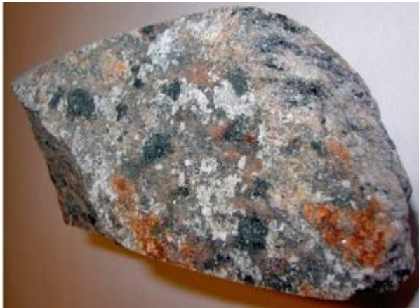
Open fracture with quartz, chlorite, corrensite, baryte and pyrite. The diameter of the drill core is c 5 cm.
