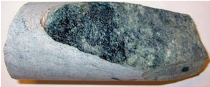
Open fracture coated with mainly chlorite/corrensite and laumontite.
