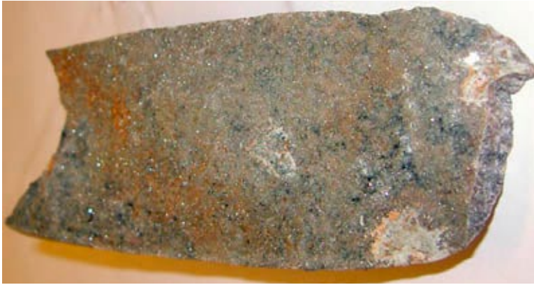
Open fracture with coating of euhedral quartz, pyrite and adularia. The diameter of the drill core is c 5 cm.
