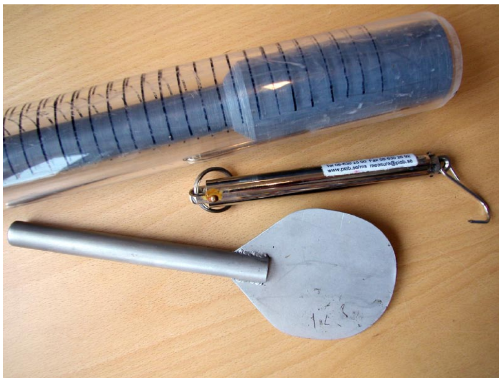
Figure 3-1. Equipment used to measure snow depth and snow weight.
