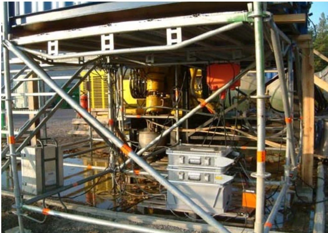
Figure 4-2. The CR23 logging unit for parameters “barometric pressure” and “electrical conductivity”.
