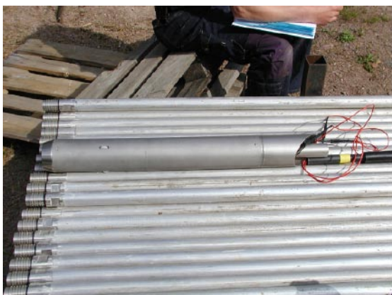
Photo 5. Positioner, bottom end of down-in-hole string.
