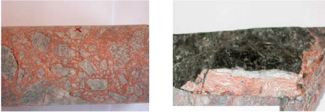
Figure 2-2. Examples of deformation zone, type 2. To the left: laumontite sealed breccia, to the right; open fracture in the deformation zone with laumontite, calcite, chlorite.
