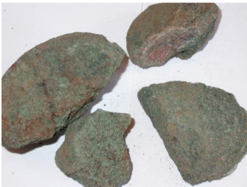
Figure 2-3. Examples of altered rock coated with chlorite and clay minerals in transmissive part of SE gently dipping brittle deformation zones.
