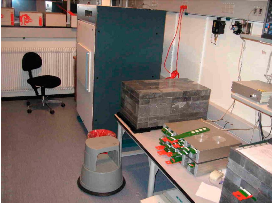
Figure 4-1. The Quantulus LSC is the cabinet shown in the background behind a set-up of the ordinary anticoincidence shielded GM gas flow counters in a lead cave in the foreground.
