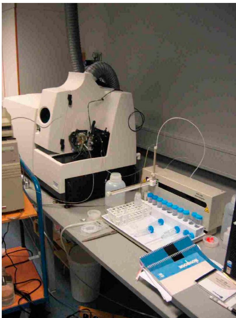
Figure 4-3. The ICP-MS system used for the analysis of Pu, Th and U isotopes.
