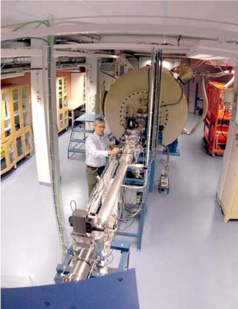
Figure 4-4. The accelerator mass spectrometer used for ^{129}\text{I} measurements.
