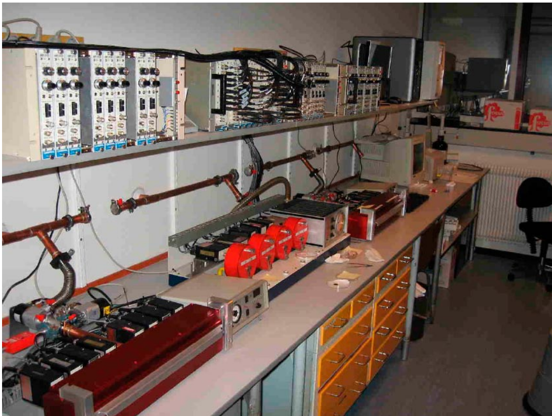
Figure 4-2. The solid state alpha spectrometry system used for the alpha spectrometry of plutonium.
