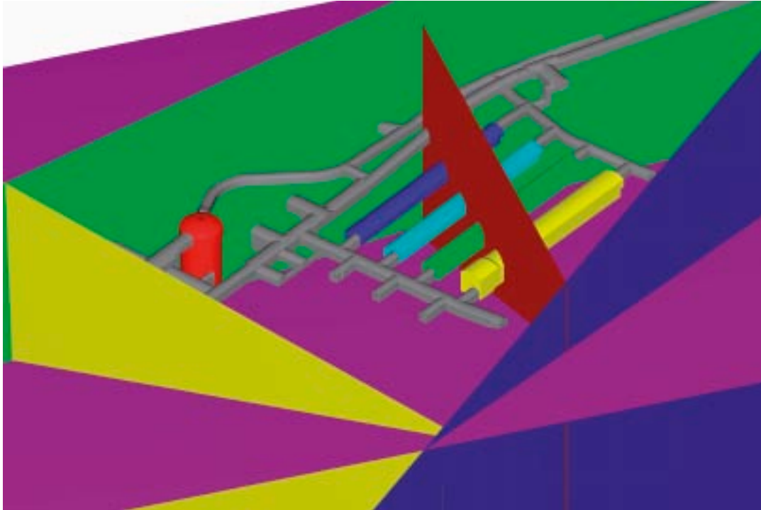
View I. A close-up view of the fracture zones and the layout of the deposition tunnels at SFR. ZONES: Purple= H2. Dark blue= 3. Dark red= 6. Yellow= 8. Green= 9. TUNNELS: Grey= Access. Red= SILO. Dark blue= BTF1. Light blue= BTF2. Green= BLA. Yellow= BMA
