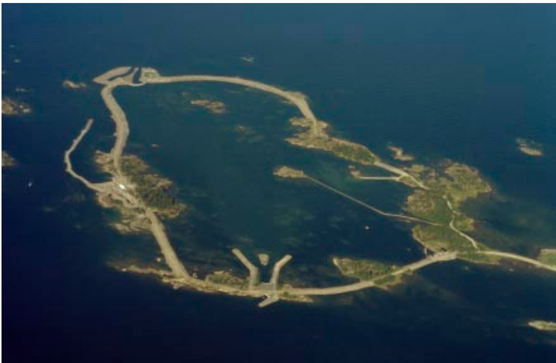
Figure 4-1. Aerial view of the bio test lake with the outlet of the Forsmark 1 and 2 tunnel in the foreground, and the outlet of the Forsmark 3 tunnel to the left (on the sea-side of the dam). Photo G Hansson/N.
