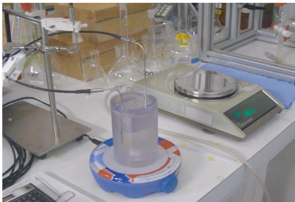
Figure 3-3. Calorimeter with two temperature sensors on magnetic stirrers.
