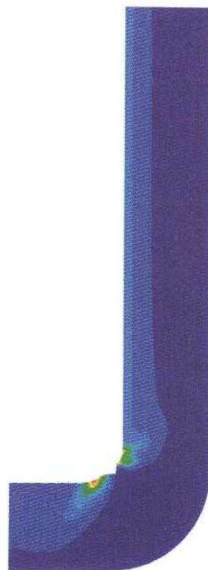
Figure 6-15: Plastic strain in bentonite for extreme global corrosion case 734550 years
