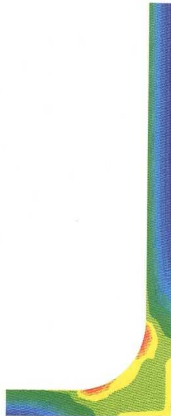
Figure 6-16: Maximum principal stress in rock for extreme global corrosion case 734550 years
