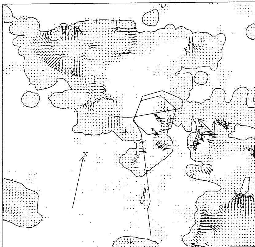
Figure 4-13. Horizontal flow at 0.25 and 4 metres depth, with complete tunnel.
