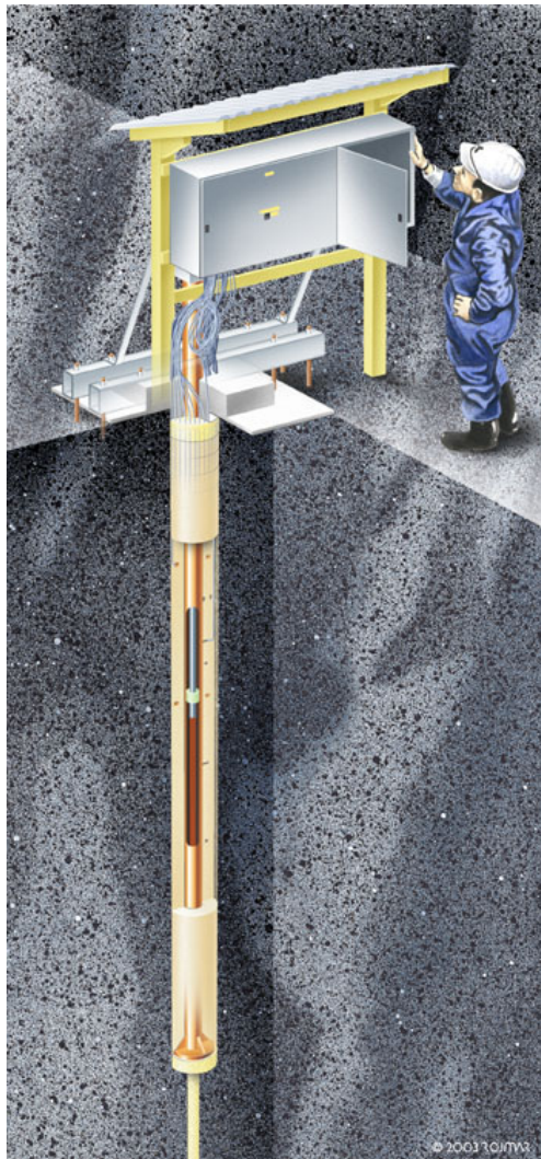
Figure 4-2 Illustration of the experimental set-up in the Long Term Test of Buffer Material (left) and a cross-section view of one S-type parcel (right).
