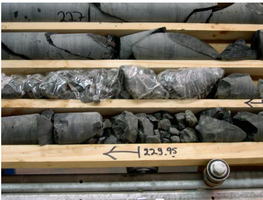
Figure 5-17. Dolerite in KLX20A. Note the strong fracturing which is characteristic along its entire length in the drill core.
