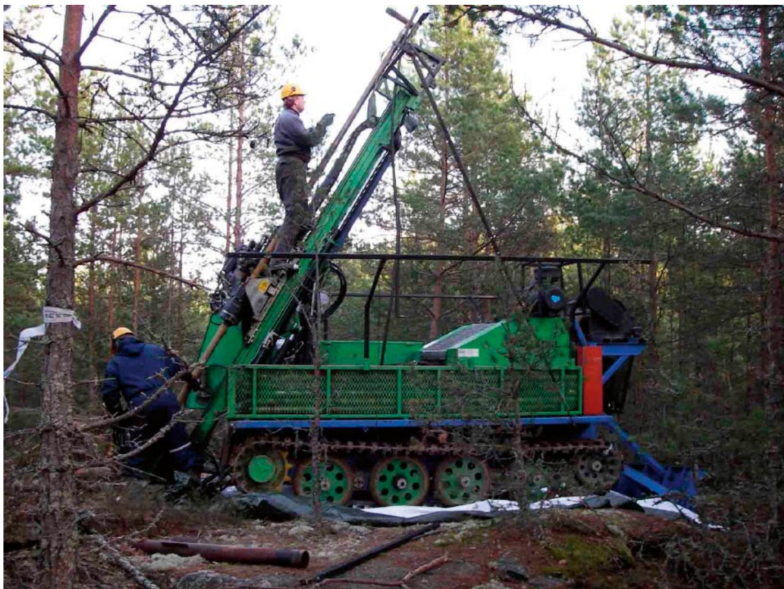
Figure 3-1. The Geomachines GM200 drill rig at KLX09E.
