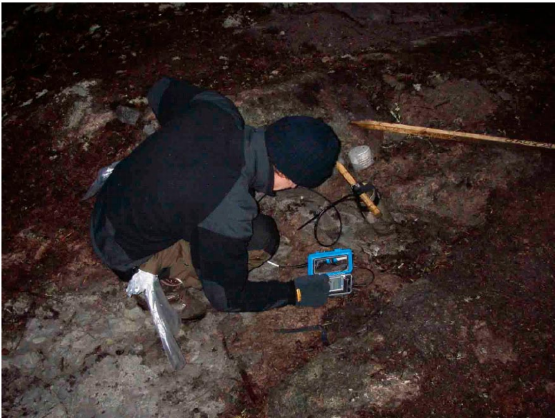
Figure 4-4. Downloading data from logger in KLX09D.
