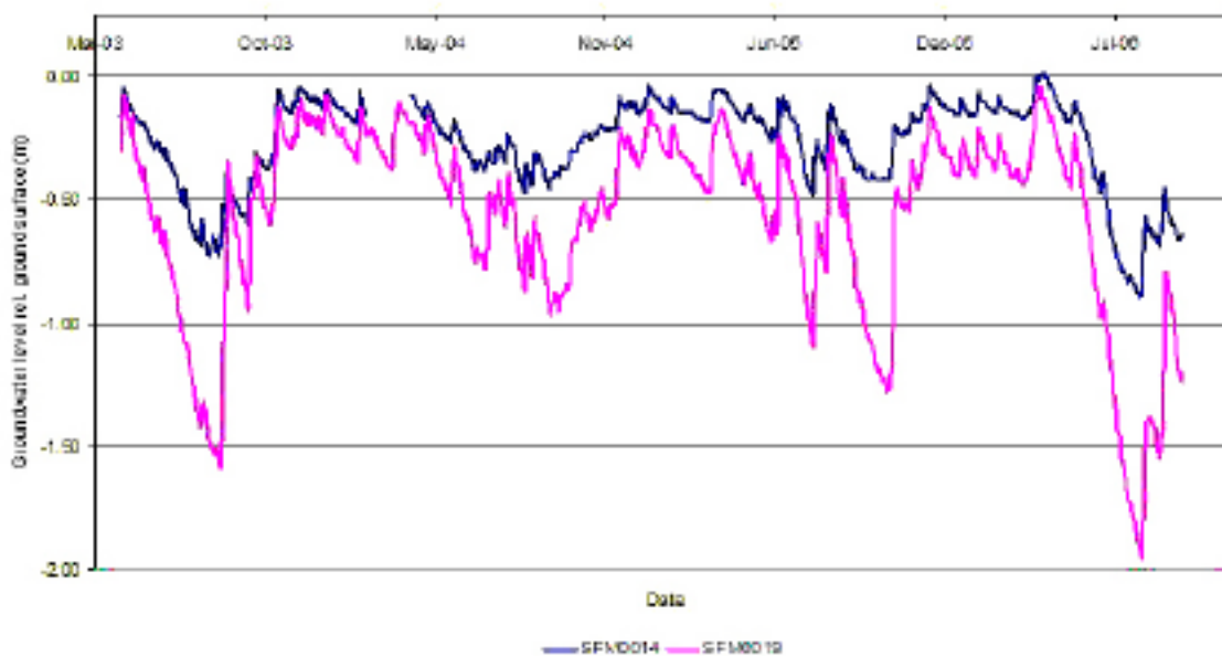
Figure 2-14. Groundwater levels in two groundwater monitoring wells in typical recharge and discharge areas, SFM0019 and SFM0014, respectively.
