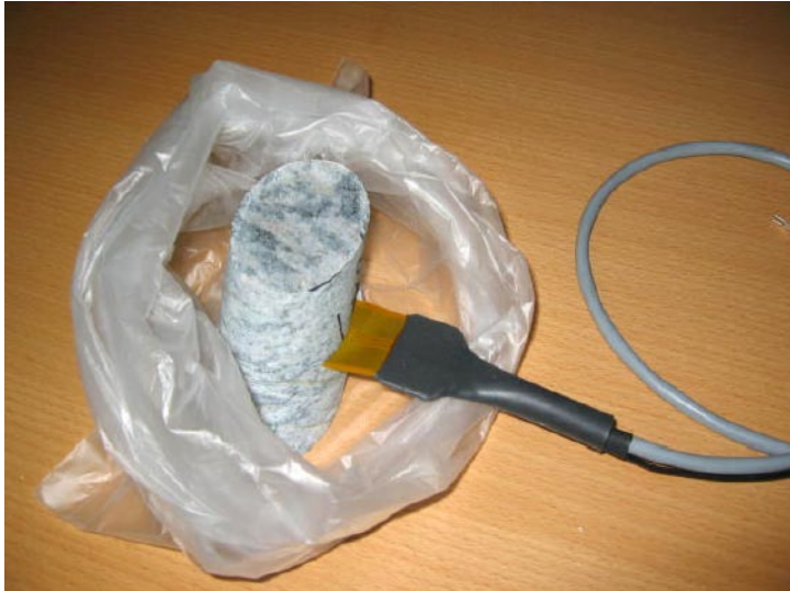
Figure 4-1. Sensor sandwiched between two sample pieces. The plastic bag was sealed off with a rubber band and a dead weight was mounted on top of the sample set-up.
