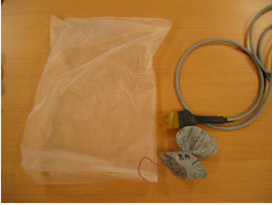
Figure 3-3. Plastic bag, rubber band sample and sensor used for the measurements in this report.
