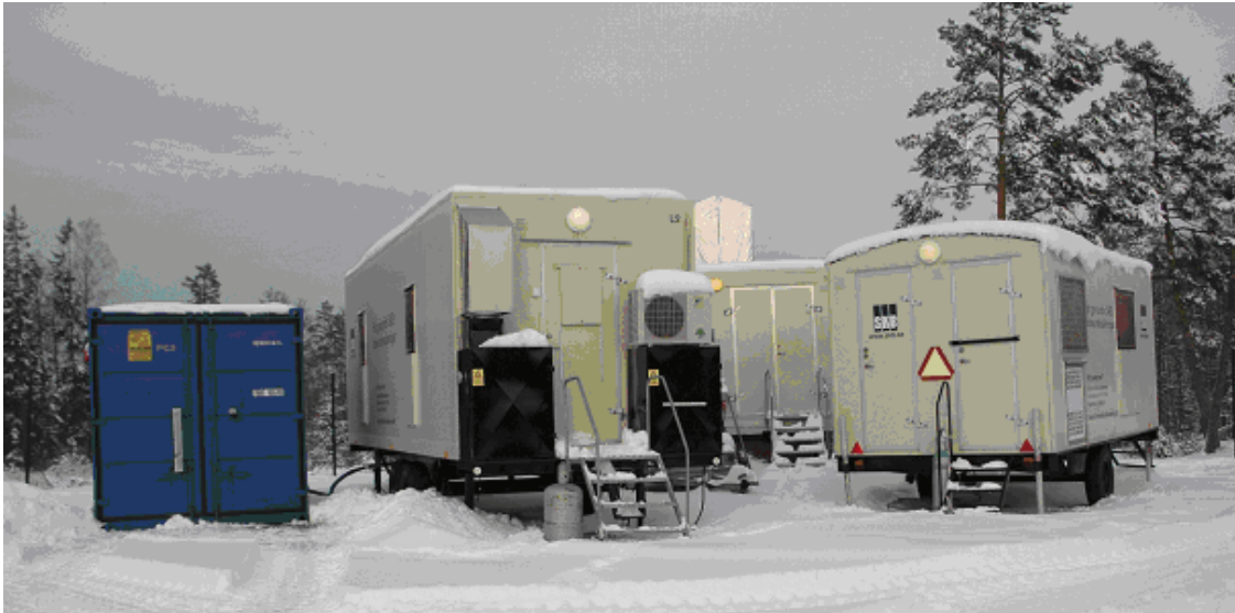
Figure 4-1. The mobile units at KLX03; from left container for collecting the water from the borehole, laboratory unit, hose unit with downhole equipment and a unit for computer work, January 2005.
