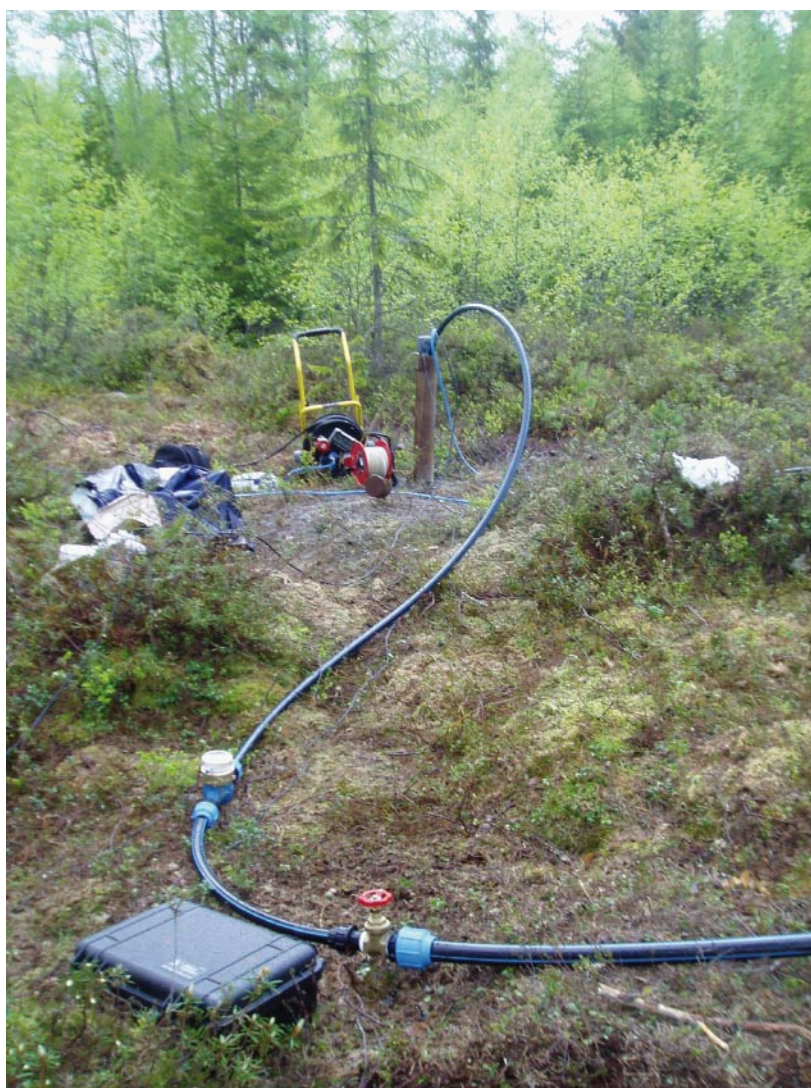
Figure 5-1. Pumping well (SFM0103), flow meter, and hose for discharge of water from the well to the recipient.
