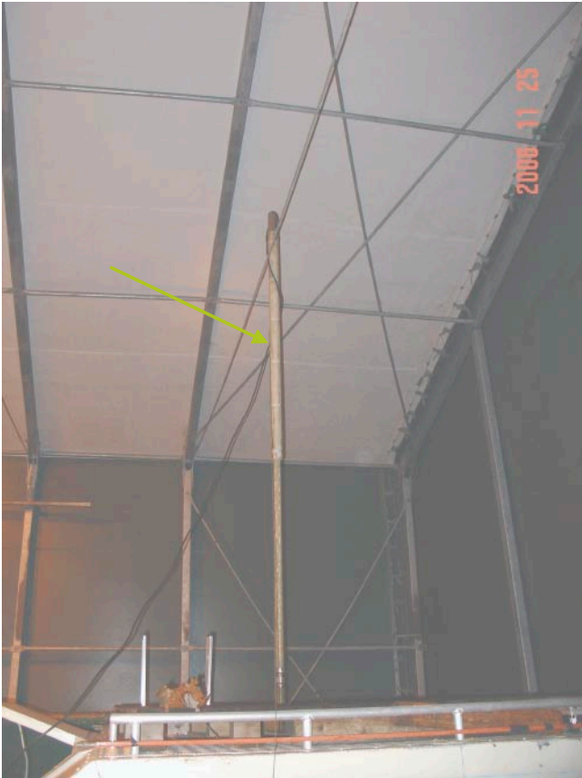
Figure 4-2. Photo of the surroundings during the functionality test of the directional antenna. The receiver antenna is seen in the middle of the picture, very close to a steel cable.
