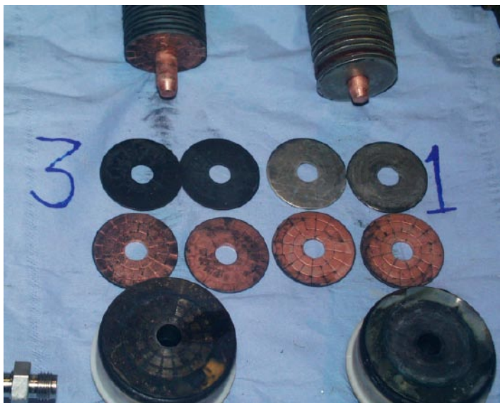
Figure 2-18. Appearance of specimens from Cells 1 (stainless steel control) and 3 (carbon steel) after exposure to artificial groundwater for 380 days at 69°C (first series). The stack of specimens can be seen at the top and the cell end plugs at the bottom.
