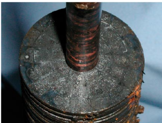
Figure 2-20. Aerated stress cell test with demineralised water, 69°C, second series of experiments, Cell 1.
