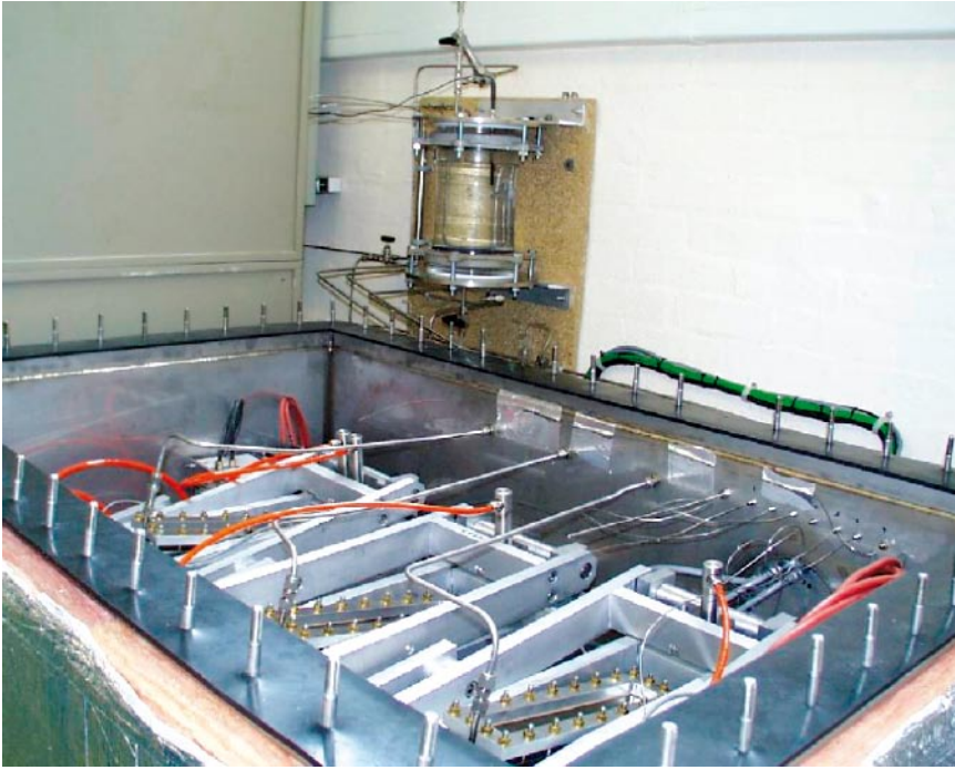
Figure 2-4. Three stress cells inside the environmental chamber, with the fluid reservoir in the background.
