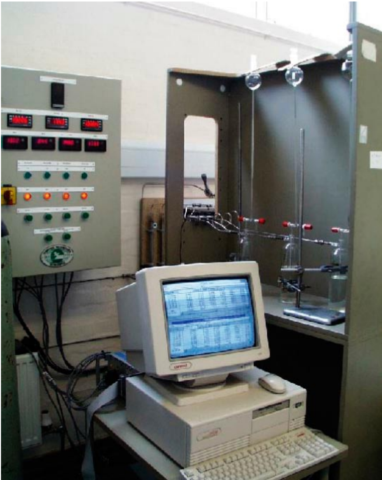
Figure 2-5. Control panel, datalogging system and manometers for stress cells.
