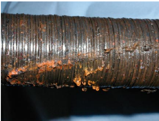
Figure 2-19. Appearance of test stack at end of experiment with cast iron (Cell 1, second series of tests).
