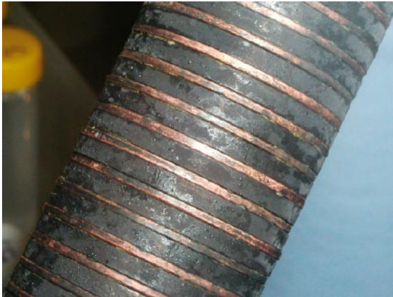
Figure 2-19. Appearance of test stack at end of experiment with cast iron (Cell 1, second series of tests).
