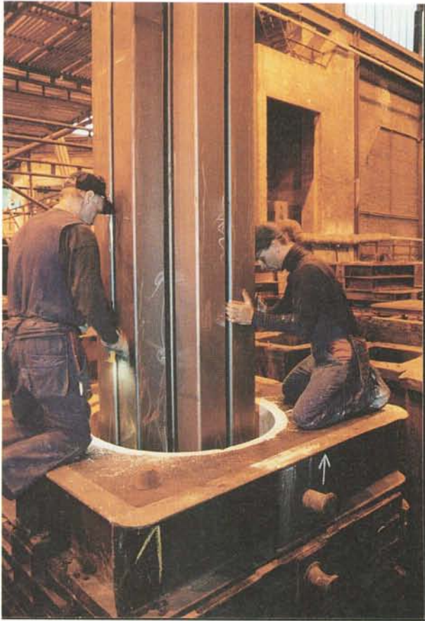
Figure 12.3-5. Preparation before casting of insert. The cassette of steel-profiles is being placed in the mould.
