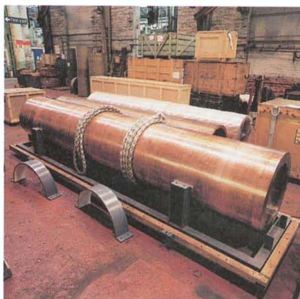
Figure 12.3-1. The first full-scale canister produced during fabrication trials.
