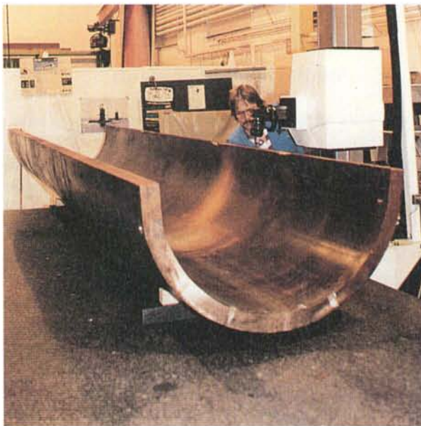
Figure 12.3-3. Dimensional check of half-cylinder before final machining.
