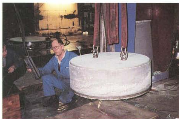
Figure 15.2-3. Compaction of cylindrical bentonite blocks with the diameter 1 meter in the press in Ystad. The upper picture shows the form and the press and the lower picture shows the compacted block.
