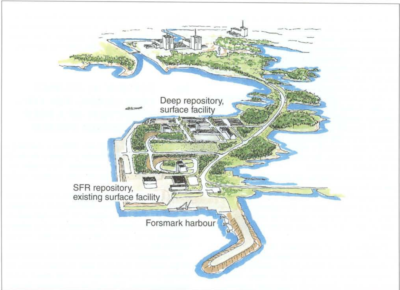
Figure 5-5. An artist view of how the surface facilities of the deep repository siting might be located besides the existing surface facility of SFR facility (final repository for radioactive operational waste). This option is feasible if the underground part of deep repository is located within 10 km from the Forsmark nuclear power plant.
