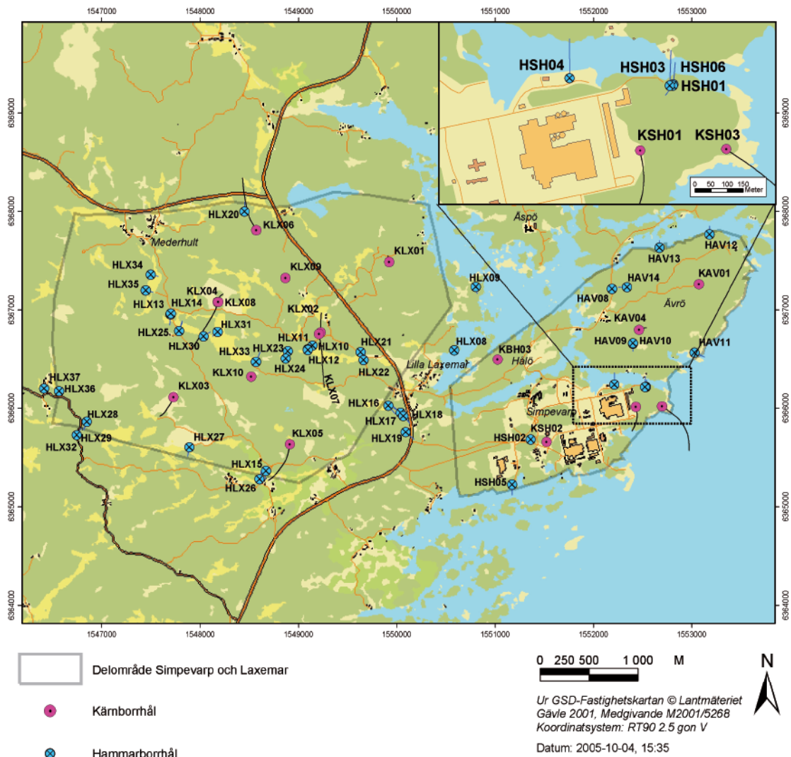
Figure 1-1. Location of all telescopic boreholes drilled up to October 2005 within or close to the Oskarshamn candidate area. The projection of each borehole on the horizontal plane at top of casing is also shown in the figure.
