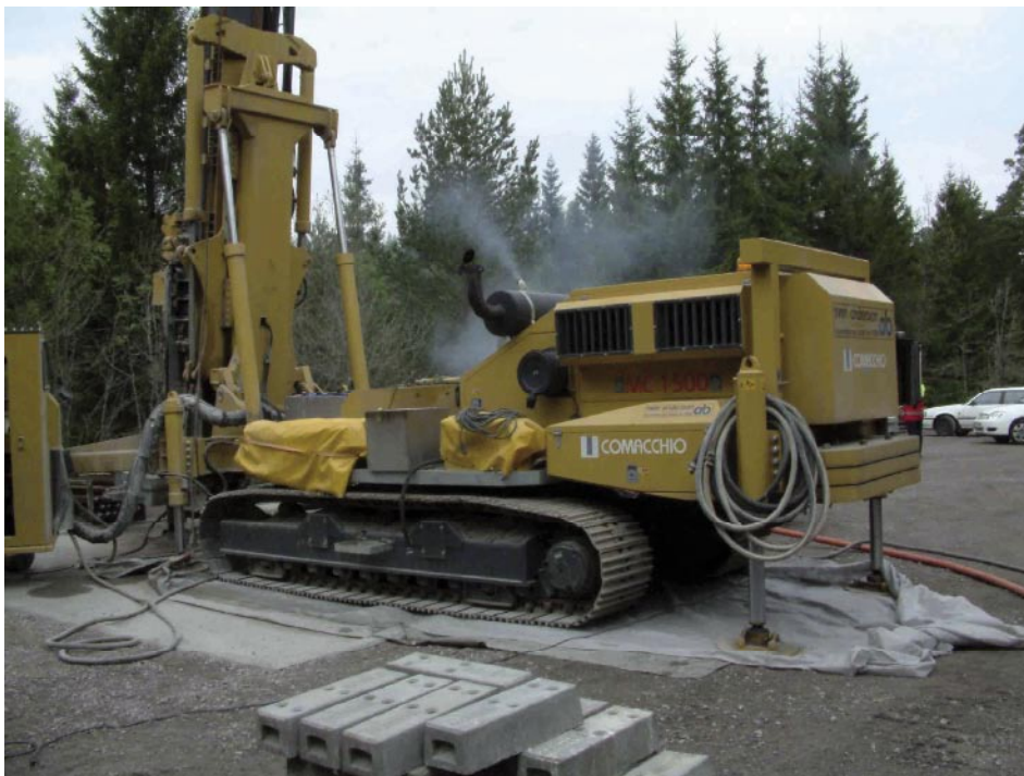
Figure 4-1. The Comacchio MC1500 percussion drill rig at KLX10.
