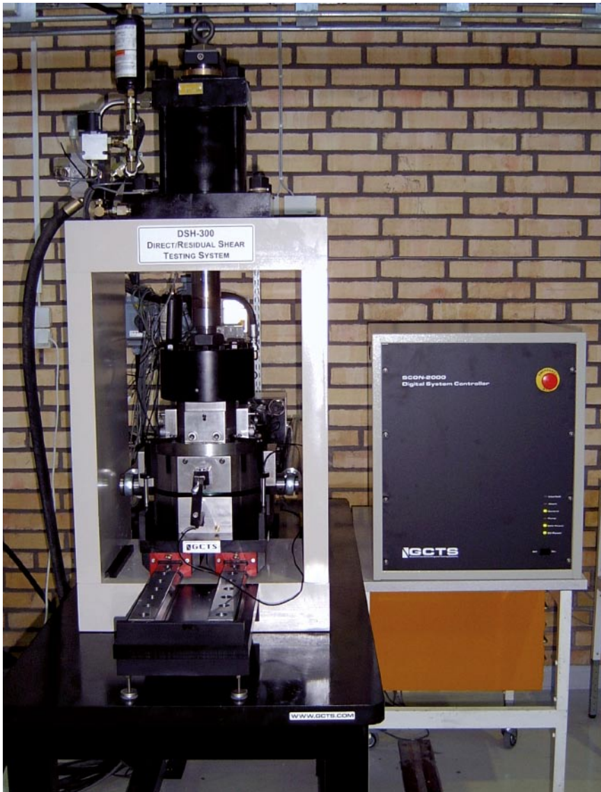
Figure 3-1. Equipment for direct shear tests and digital controller unit.
