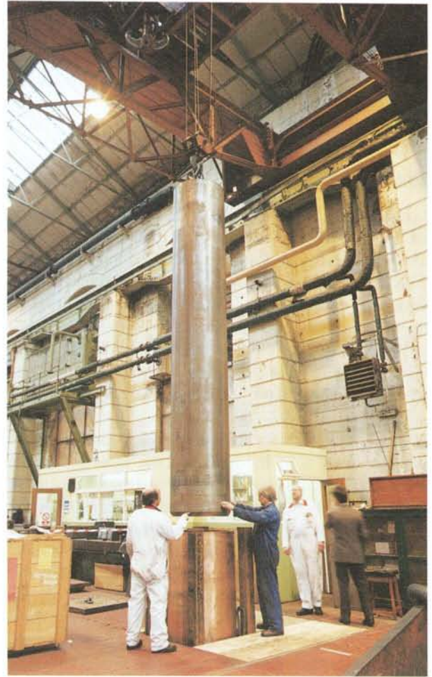
Figure 13-3. Assembling of copper cylinder and steel insert.
