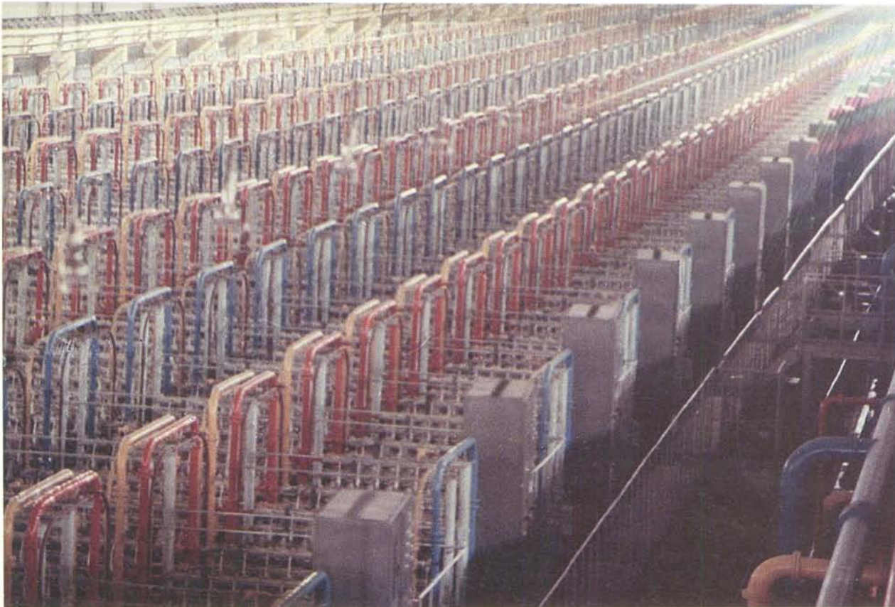
Figure 9-2. Gas centrifuges in the Ural Electrochemical Integrated Plant for enrichment of uranium.
