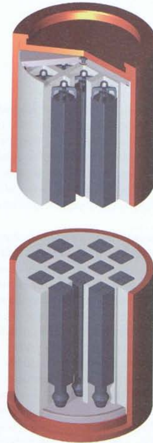
Figure 6-1. Copper canister with cast insert.
