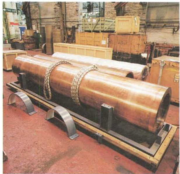
Figure 13-2. The first full-scale canister produced during fabrication trials.
