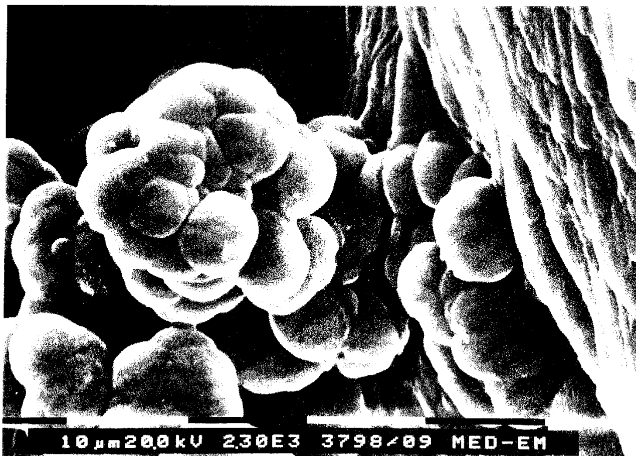
Figure 16.2-1. CSH substances from the 16 month percolation test with a solution pH of 13.5. The material is concentrated by evaporation of the bentonite percolating water, and examined by use of scanning electron microscopy. The silica-calcium ratio in this sample is around 3. The magnification is 2300 times.
