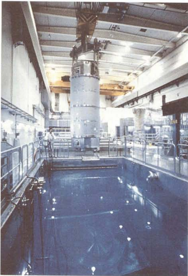
Figure 2-2. Fuel cask with protective shirt being moved from the cooling cell to the unloading pool.
