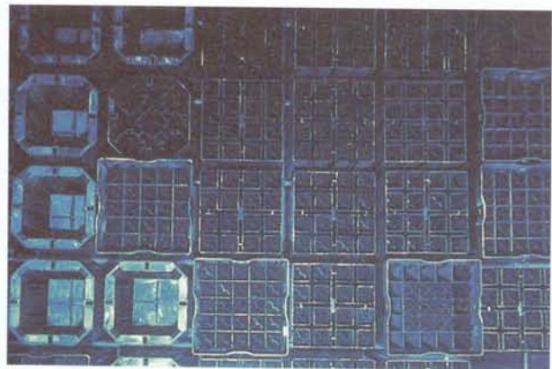
Figure 2-3. BWR-fuel canister of the old and new types containing 16 respectively 25 fuel assemblies. The octagonal canisters are used for highly radioactive reactor core components.
