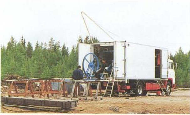
Figure 10-2. Equipment for rock stress measurements, which have been carried out on behalf of TVO in Finland.
