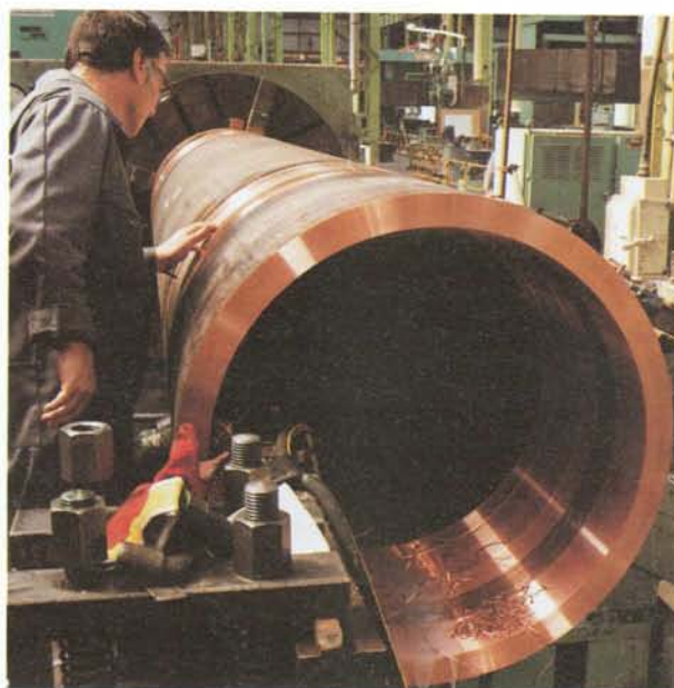
Figure 6-2. Machining of copper cylinder with 50 mm wall thickness.
