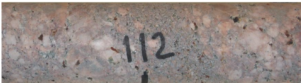
Figure 5-3. Altered vuggy pegmatite, 112 m borehole length. Scale 5:7.
