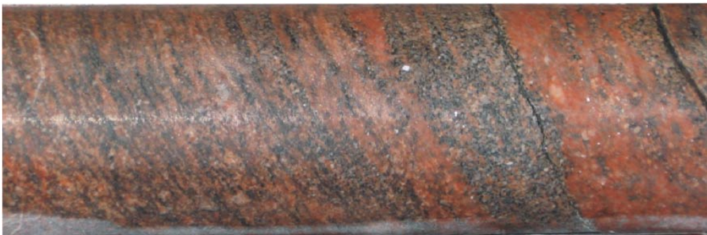
Figure 5-2. Metagranite to granodiorite showing relatively high strain, 71 m borehole length. Scale 9:10.
