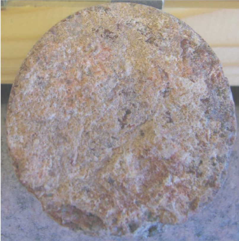
Figure 5-1. Typical fracture mineral filling in the interval 478–488 m borehole length.
