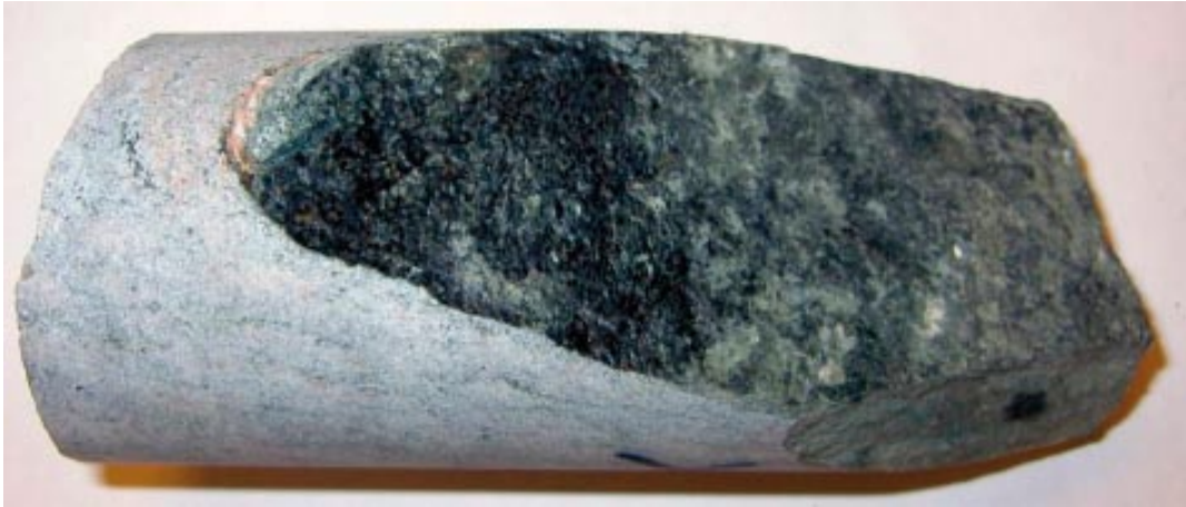
Figure 2-9. Chlorite coated fracture. The diameter of the drill core is ~ 5 cm (KFM07A 118.18–118.35 m).
