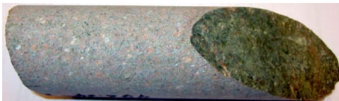
Figure 3-14. Chlorite coated fracture. Drill core diameter is \sim 50 mm (KSH03A: 452.36 m).
