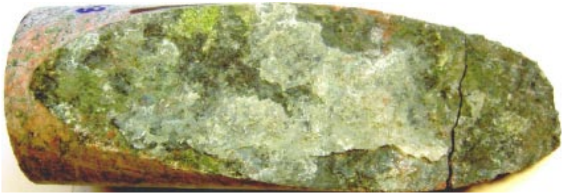
Figure 3-15. Calcite coated fracture. Drill core diameter is ~ 50 mm (KLX07A: 346.73–346.82 m).
