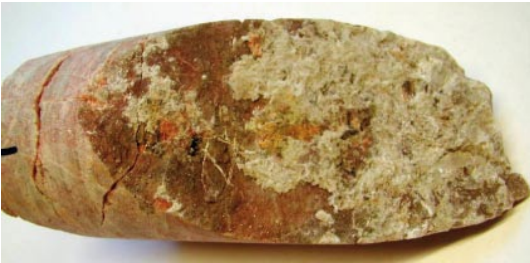
Figure 2-10. Calcite coated fracture surface. The diameter of the drill core is ~ 5 cm (KFM06A 743.39–743.52 m).
