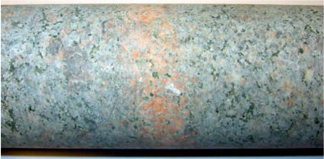
Figure 3-17. Photograph of a typical, hardly visible, sealed fracture with no visible fill but with altered wall rock. Drill core diameter is about 50 mm. These fractures are presented as “no fill – altered walls” in this report.
