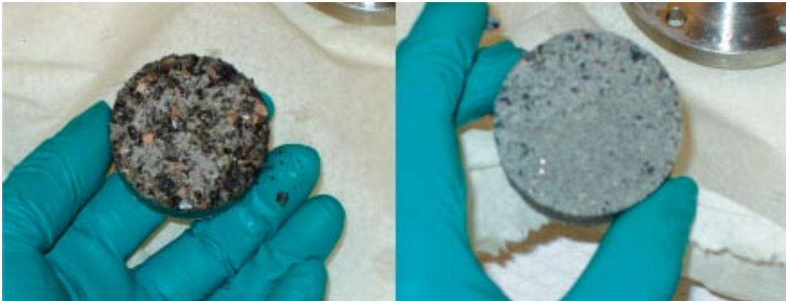
Figure 4-3. Pictures of the top and bottom of sample Mix 1:2 after dismantling.
