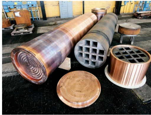
Figure 1: Canisters for spent BWR nuclear fuel. The canister consists of a cylindrical copper shell with a pressure-bearing insert of nodular iron. The outer diameter is 1.05 m and the length 4.83 m [1].
