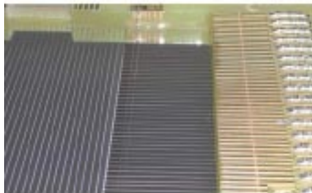
Figure 1. Detail of a CLODIA chamber on the left strips (vertical) for drift field and X localization, Strips (Horizontal) and CMS resistors for Y localization, the wire is seen near the middle of the picture
